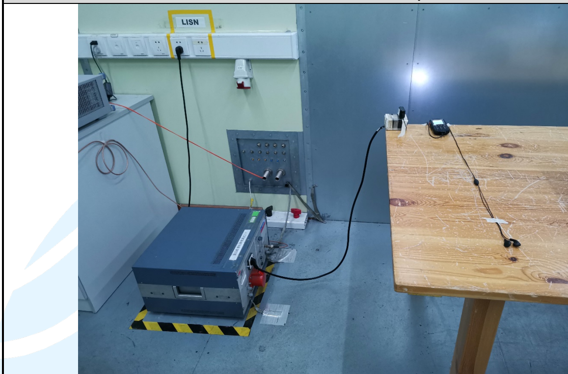
Conducted Emission Test Setup
