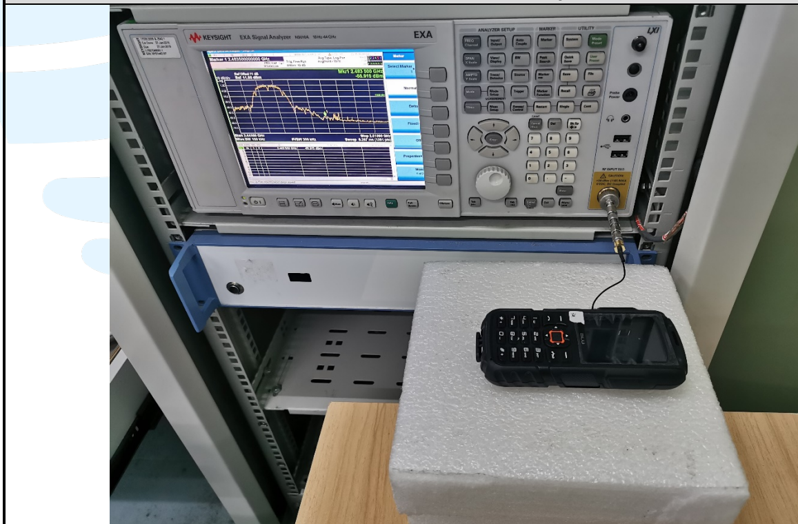
RF Conducted Test Setup
