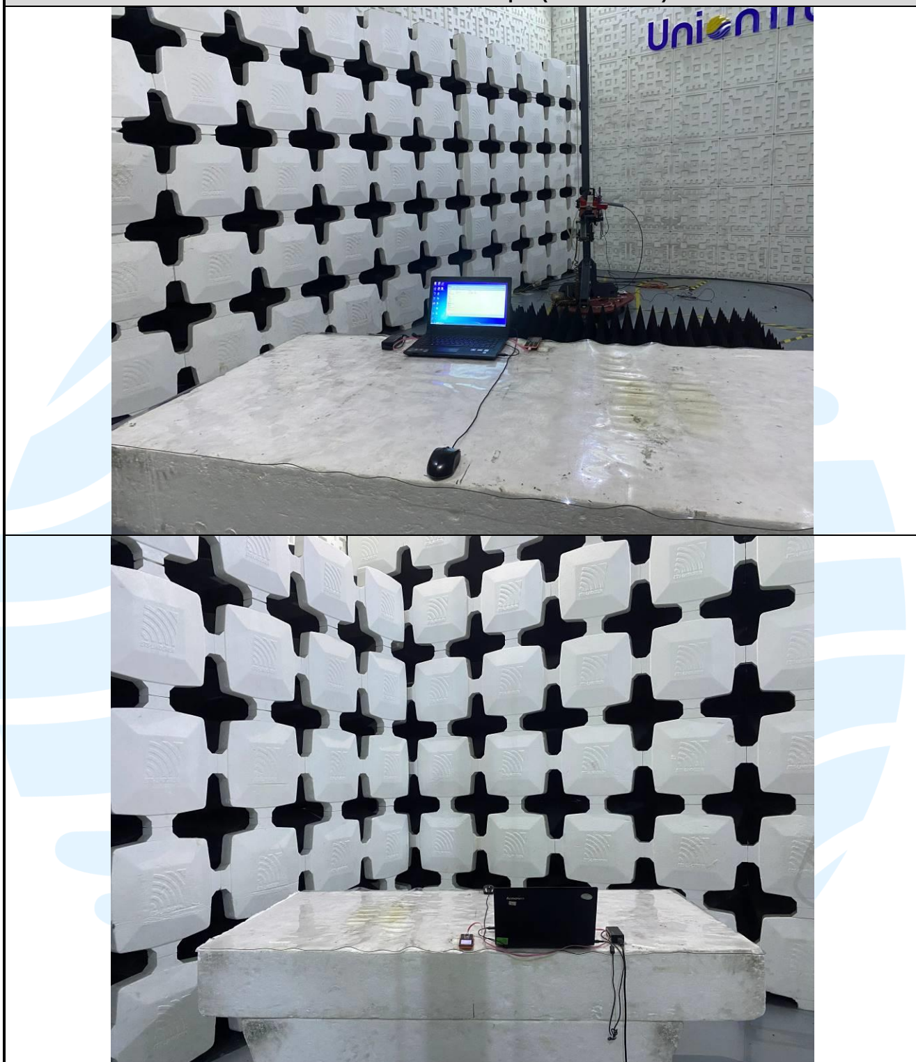
Radiated emission Test Setup-2 (Above 1 GHz)
