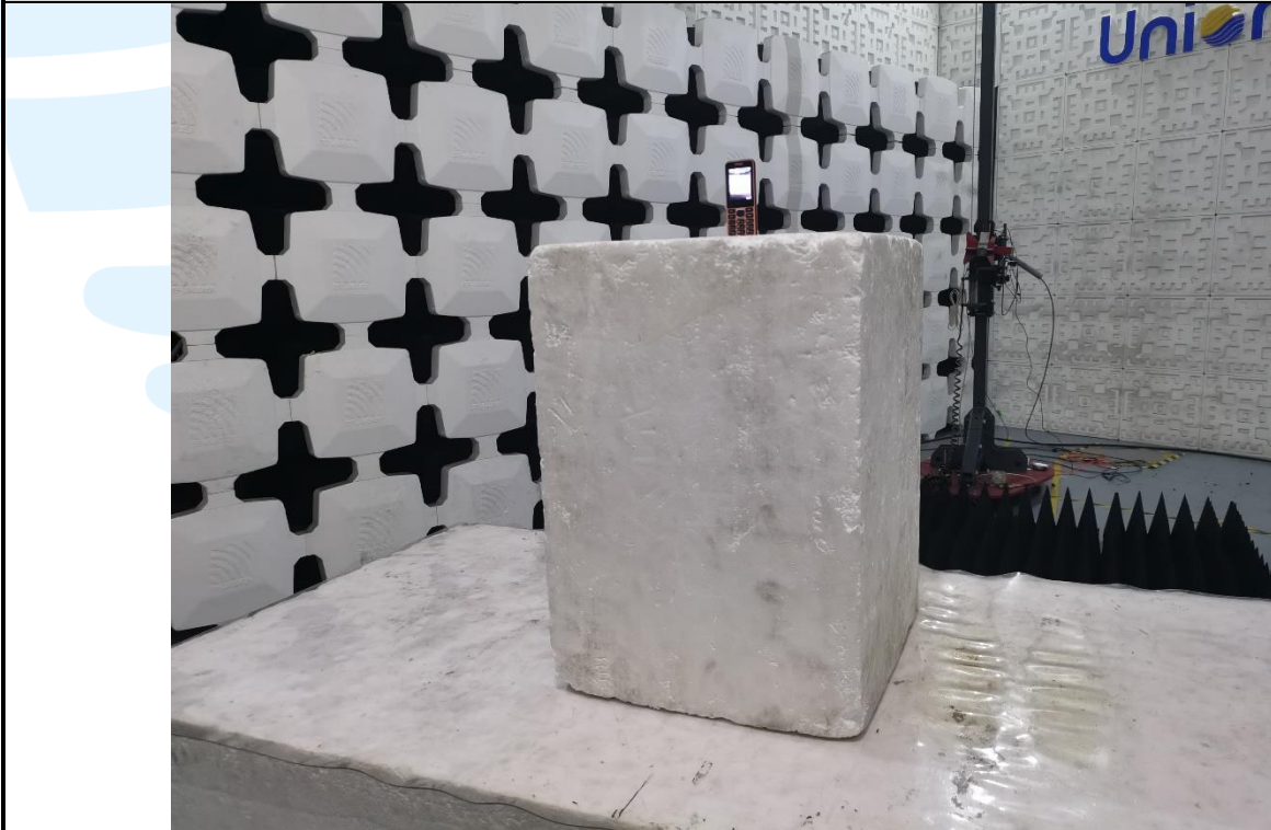
Radiated emission Test Setup (Above 1 GHz)
