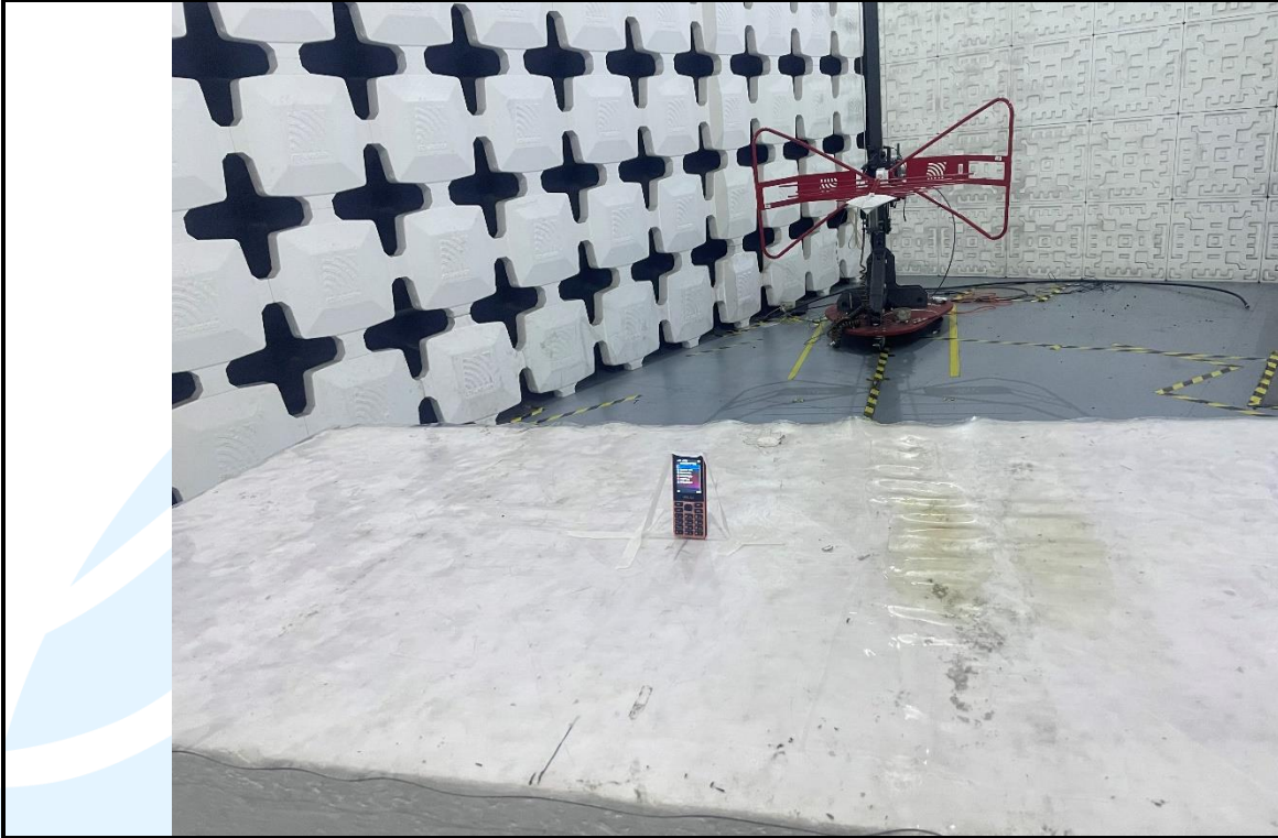
Radiated emission Test Setup (30 MHz~1 GHz)
