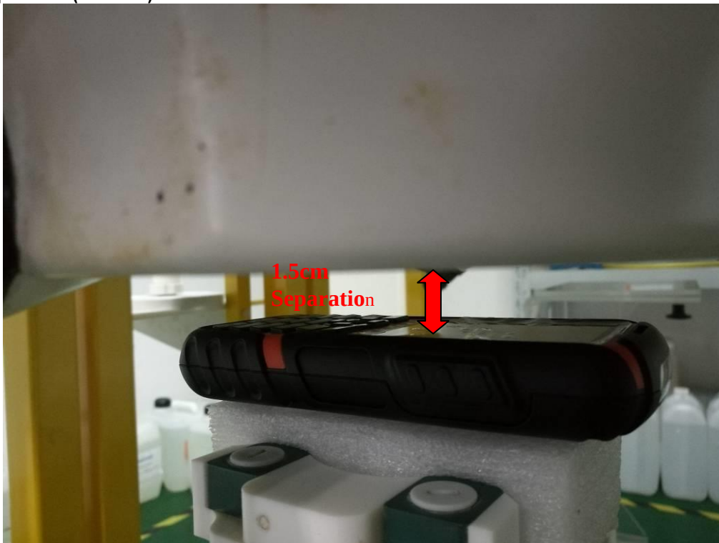
Body Setup Photo (LCD DOWN)
