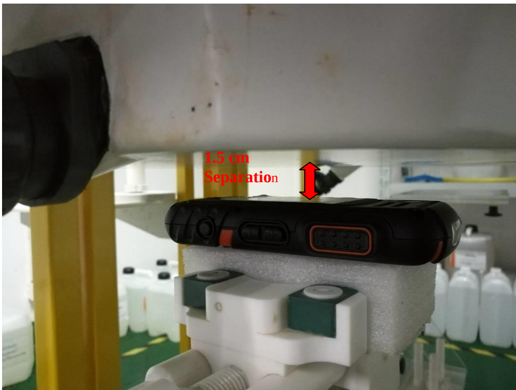
Body Setup Photo (LCD DOWN)
