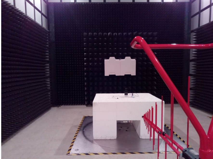
Radiated Emissions View (Below 1 GHz)
