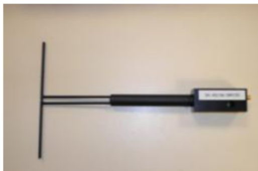
Figure 1 – Satimo COMOSAR Validation Dipole
