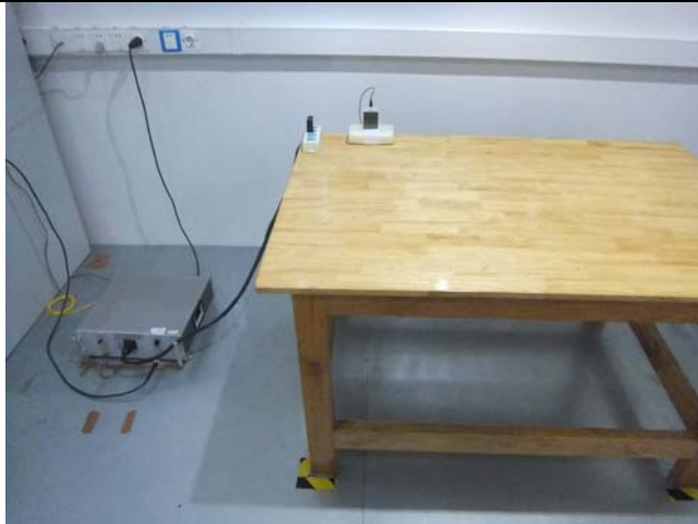
Conducted Emissions Test Setup Front View
