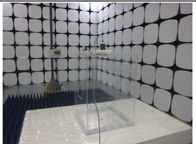
Radiated Spurious Emissions Test Setup Above 1GHz
