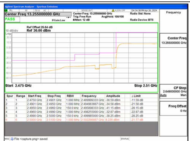
B7 / 15MHz / Low CH / QPSK / FULL RB
