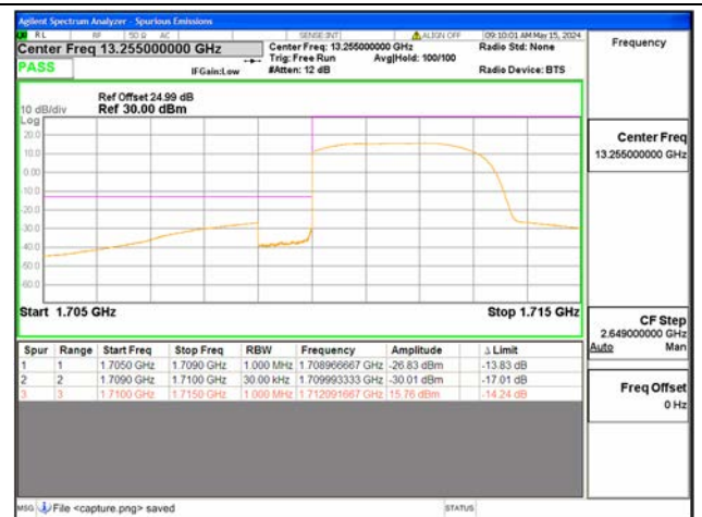
B66 / 3MHz / Low CH / QPSK / FULL RB
