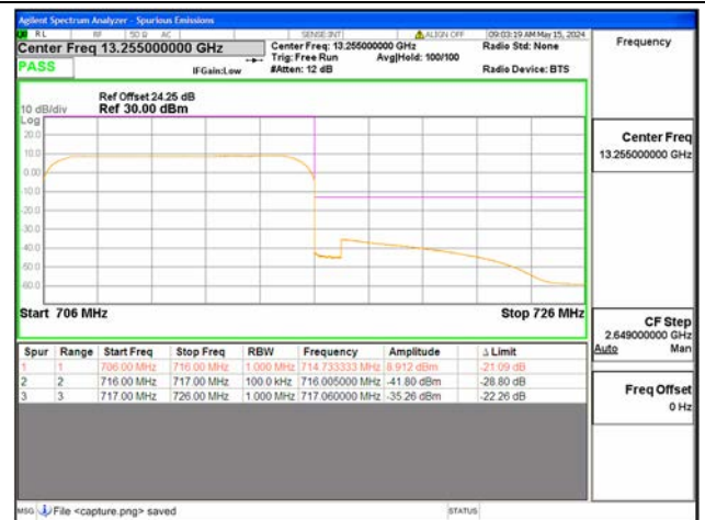
B17 / 10MHz / High CH / QPSK / FULL RB
