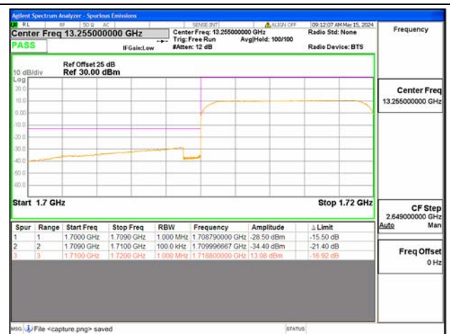
B66 / 10MHz / Low CH / QPSK / FULL RB
