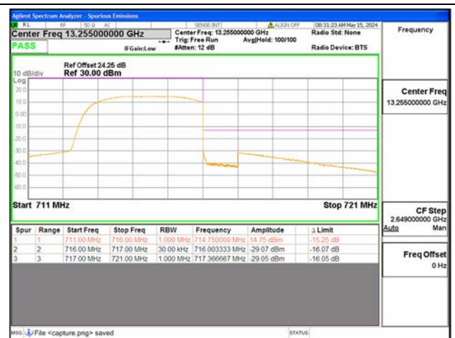
B12 / 3MHz / High CH / QPSK / FULL RB
