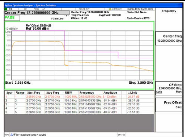
B7 / 15MHz / High CH / QPSK / FULL RB
