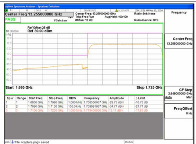
B66 / 15MHz / Low CH / QPSK / FULL RB
