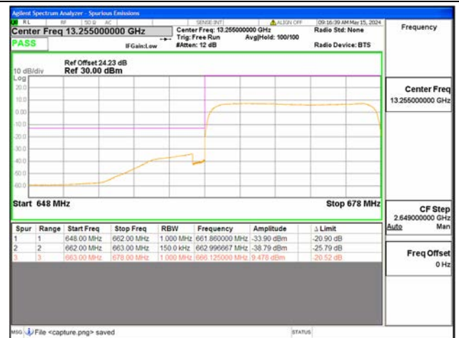
B71 / 15MHz / Low CH / QPSK / FULL RB
