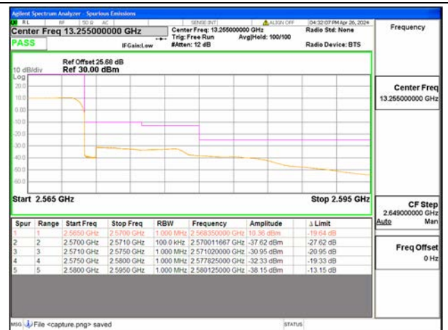
B7 / 10MHz / High CH / QPSK / FULL RB
