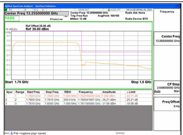
B66 / 20MHz / High CH / QPSK / FULL RB
