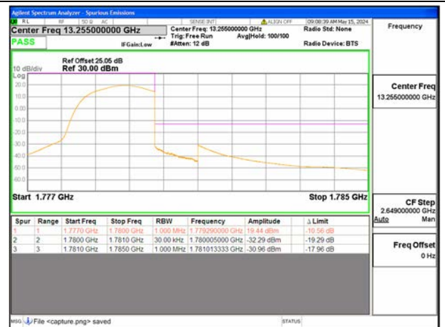
B66 / 1.4MHz / High CH / QPSK / FULL RB
