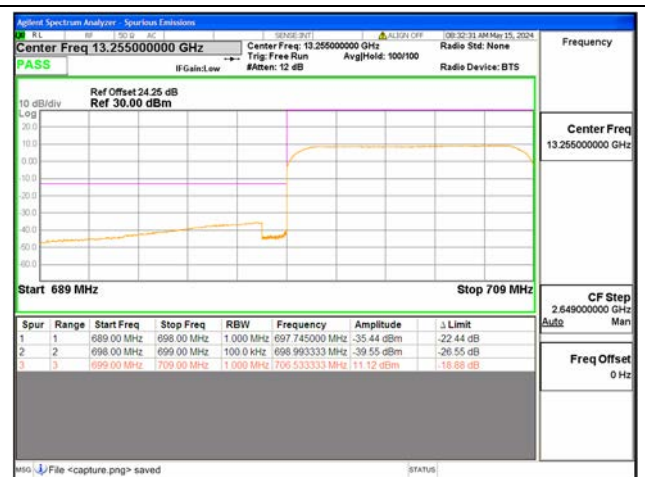
B12 / 10MHz / Low CH / QPSK / FULL RB
