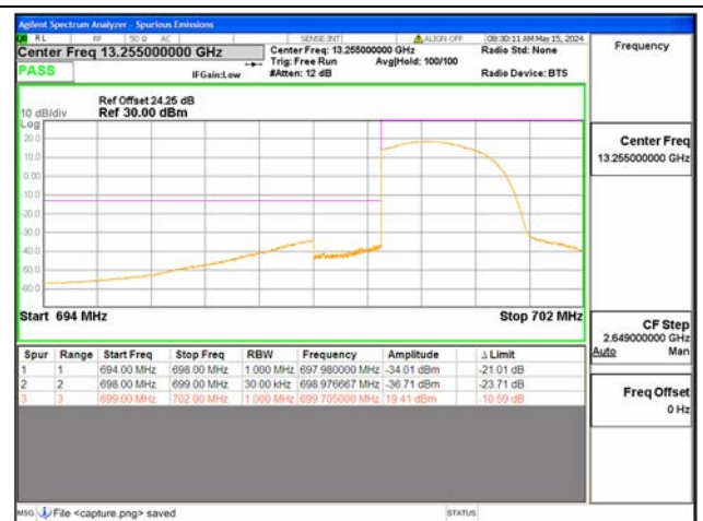
B12 / 1.4MHz / Low CH / QPSK / FULL RB
