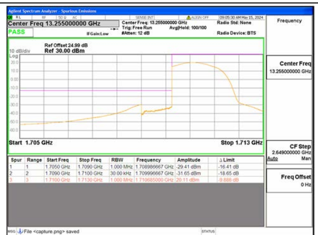
B66 / 1.4MHz / Low CH / QPSK / FULL RB
