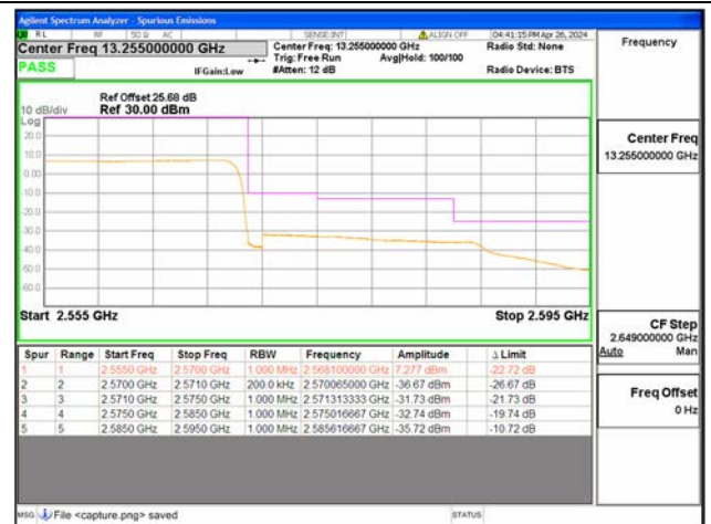
B7 / 20MHz / High CH / QPSK / FULL RB
