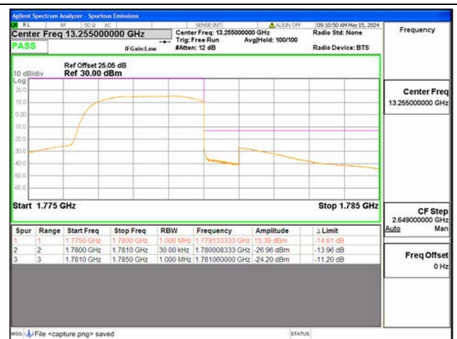
B66 / 3MHz / High CH / QPSK / FULL RB
