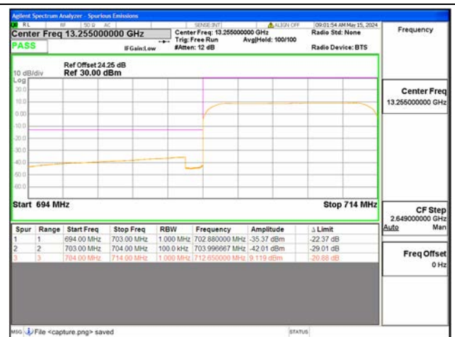
B17 / 10MHz / Low CH / QPSK / FULL RB
