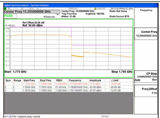
B66 / 5MHz / High CH / QPSK / FULL RB
