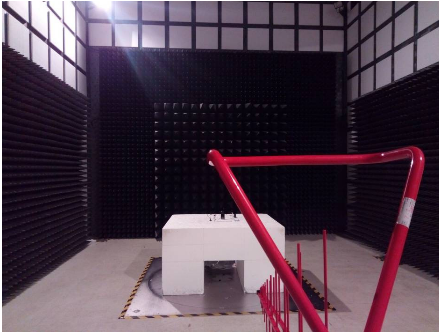
Radiated Emissions View (Below 1 GHz)
