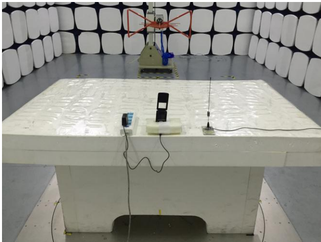
Radiated Spurious Emissions Test Setup Below 1GHz
