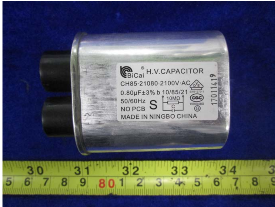
EUT –H.V. CAPACITOR View
