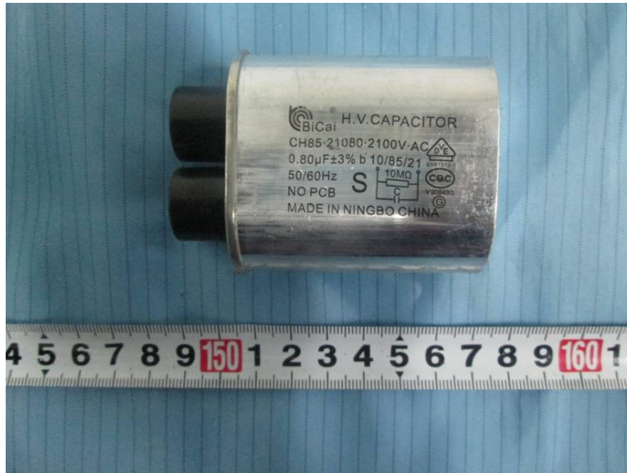
EUT – High Voltage Capacitor Top View
