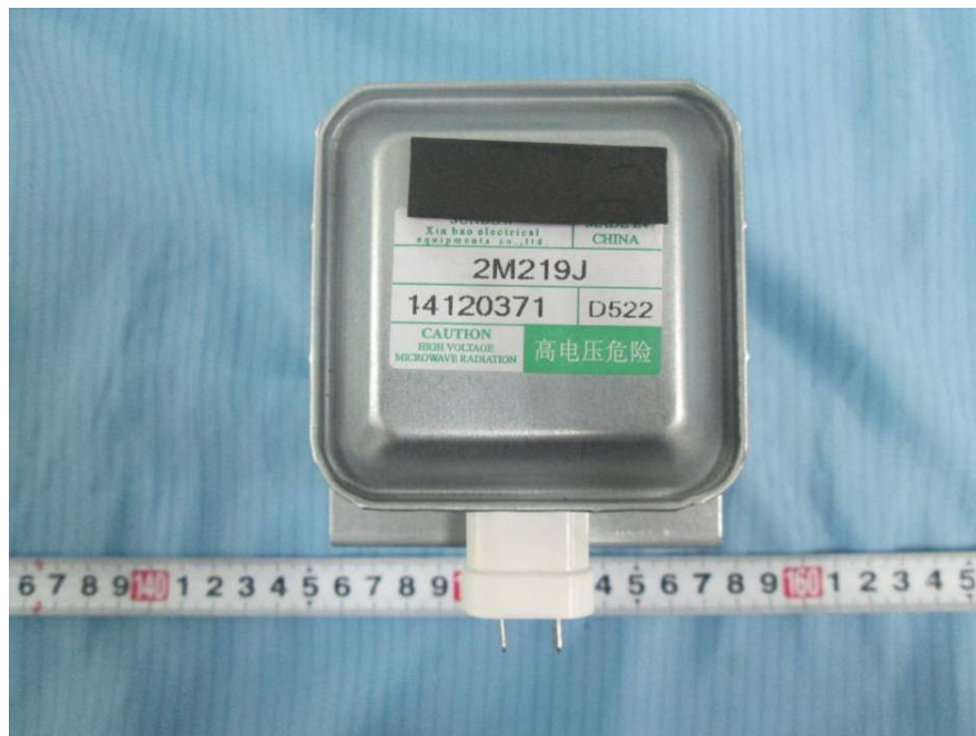
EUT – Magnetron Top View
