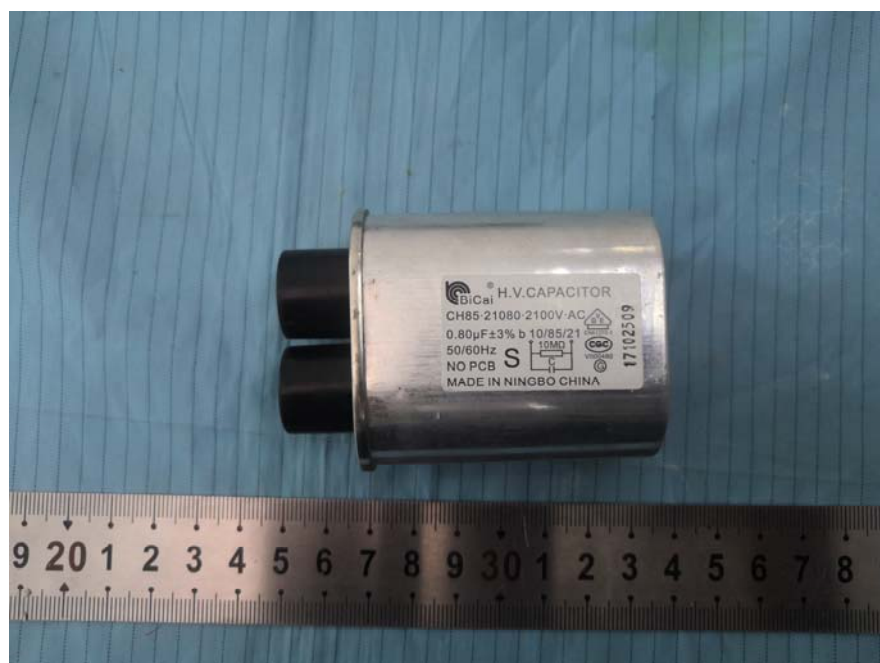
EUT – H.V. CAPACITOR Front View
