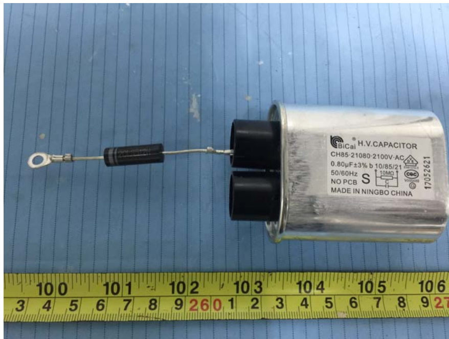
EUT – H.V. CAPACITOR & Diode View
