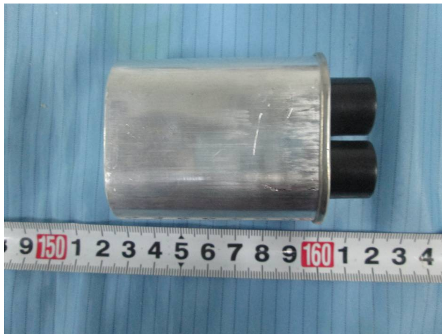
EUT –High Voltage Capacitor Bottom View
