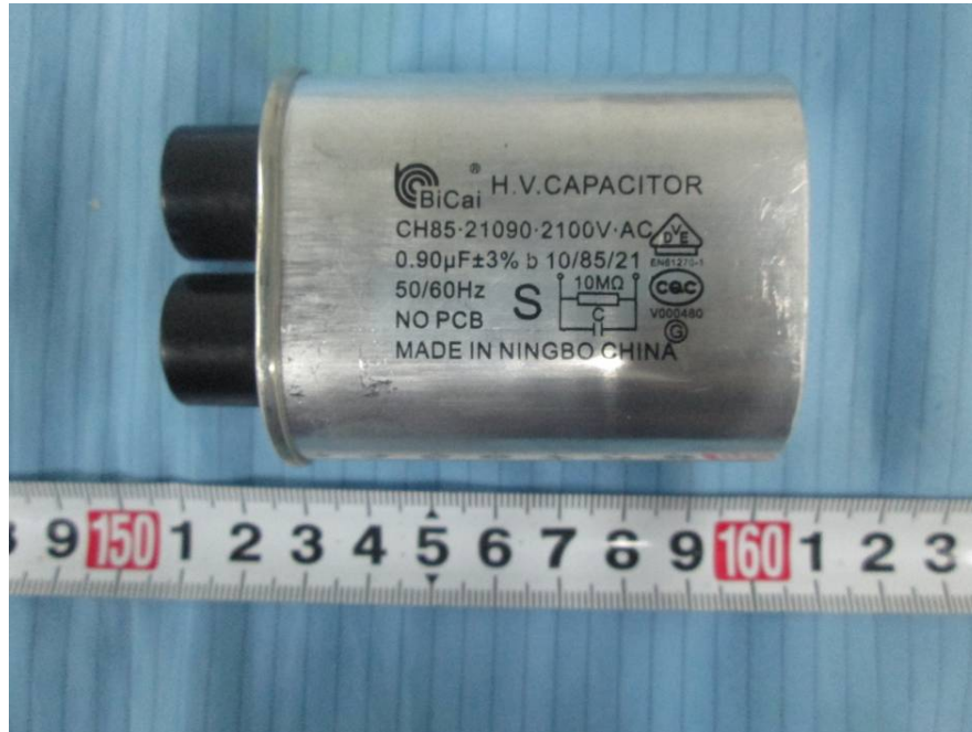
EUT – High Voltage Capacitor Top View
