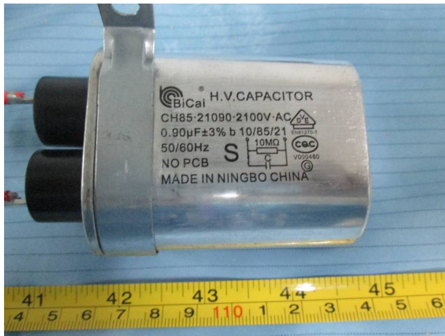
EUT – H.V. Capacitor View
