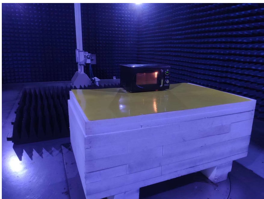
Photo of Radiation Emission Measurement- Above 1GHz
