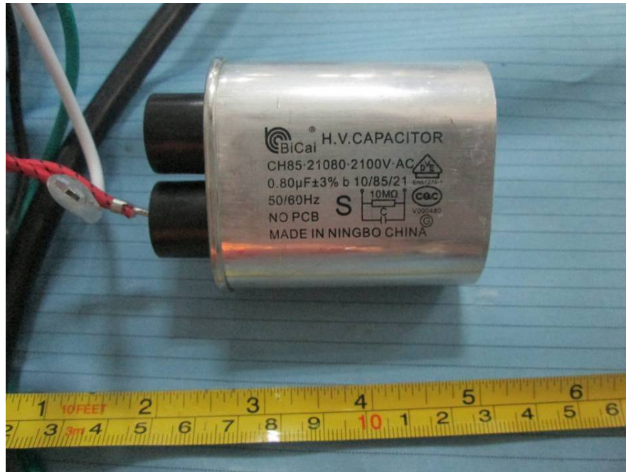
EUT –H.V. Capacitor View
