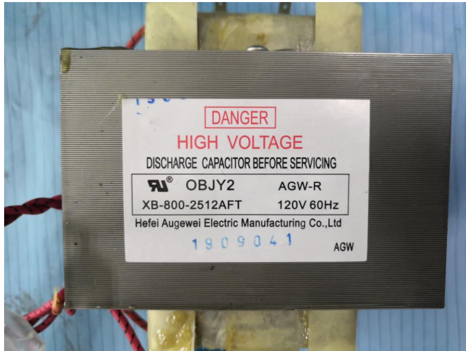
EUT – Transformer Label View
