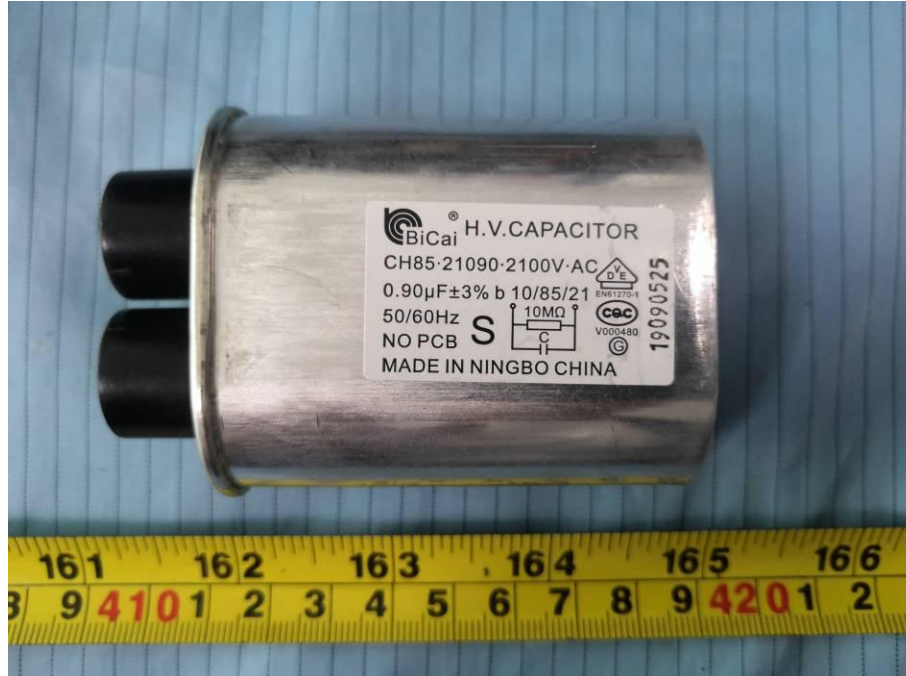
EUT – H.V. Capacitor Top View
