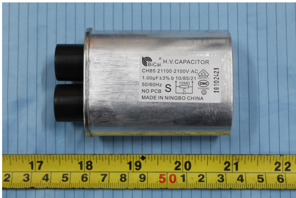
EUT – H.V. Capacitor View
