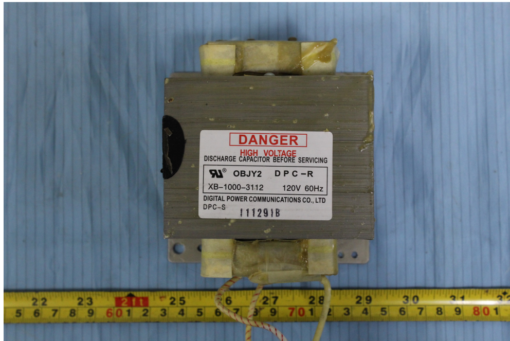
EUT – Transformer View
