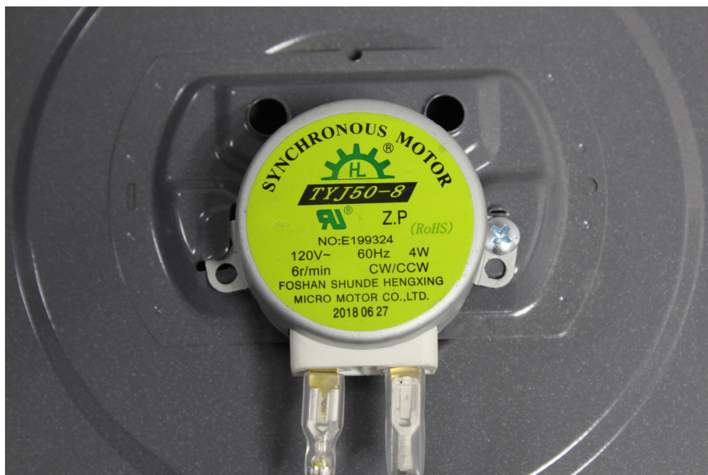
EUT –Synchronous Motor View
