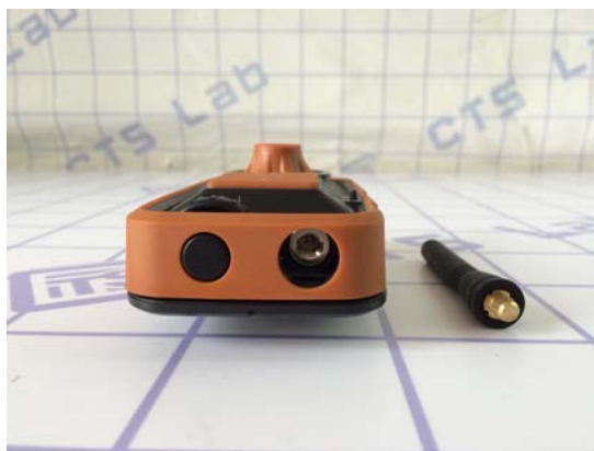
Antenna port view
