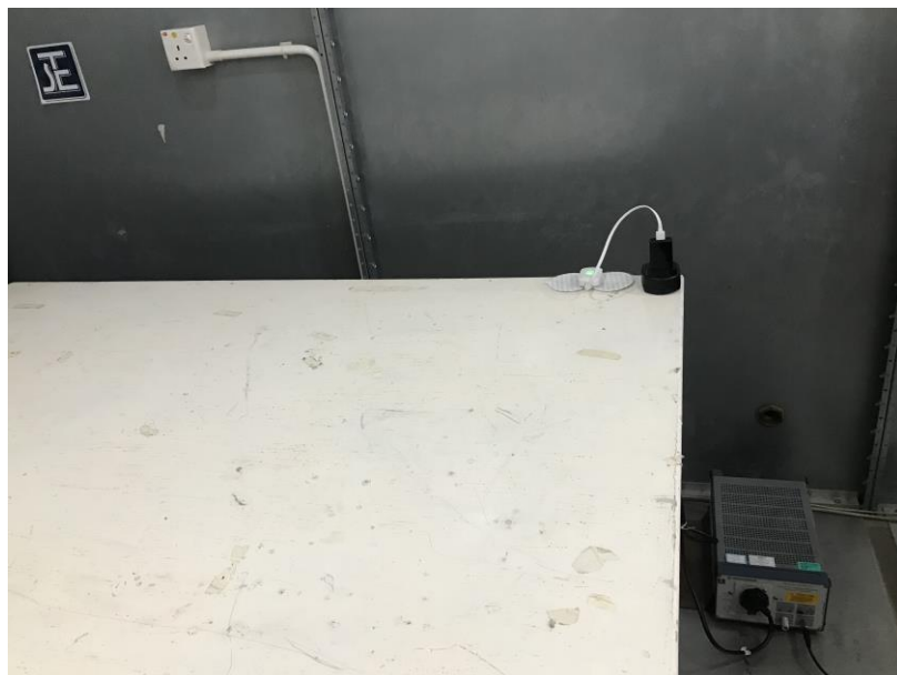
Measurement of Conducted Emission Test Set Up
