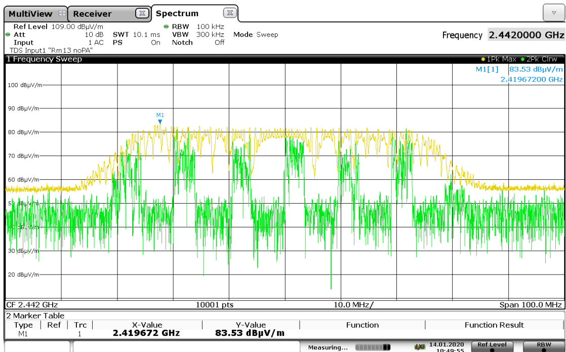
Graph 6-9: 100 kHz bandwidth reference level, 22 MHz Bandwidth
