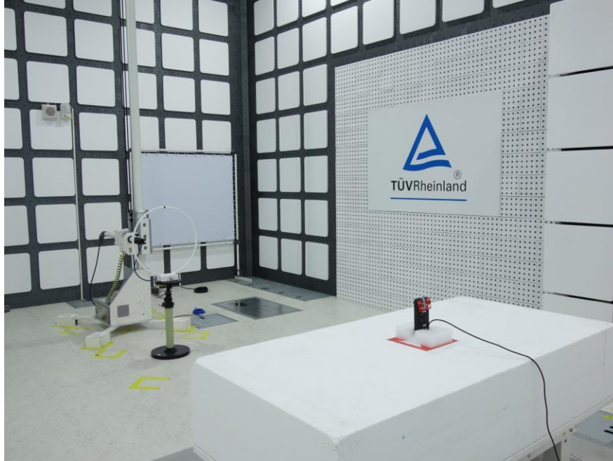
Photograph 3: Test Setup for Spurious Emissions (Back View 1)
