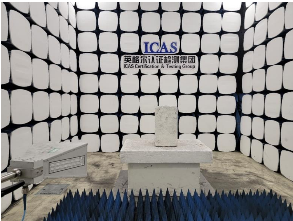
FCC Radiated Emission Test Setup-above 1GHz
