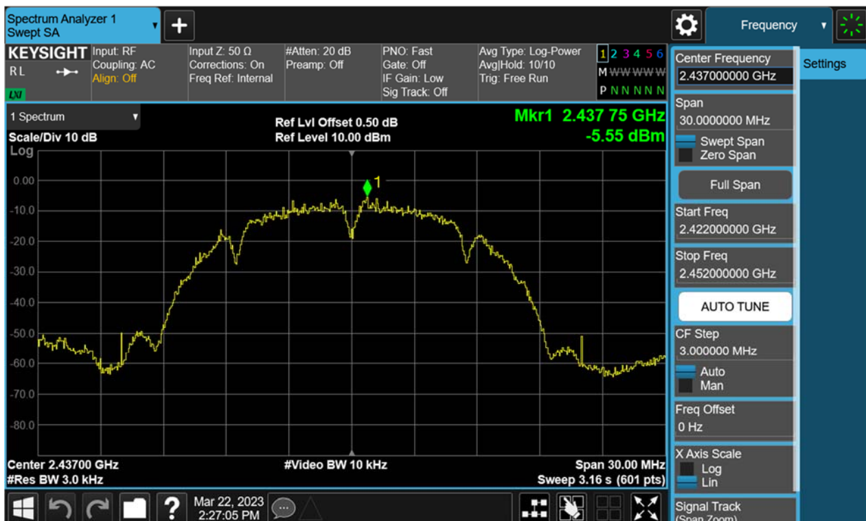
Figure 14: Power Spectral Density, 802.11b, 2437MHz
