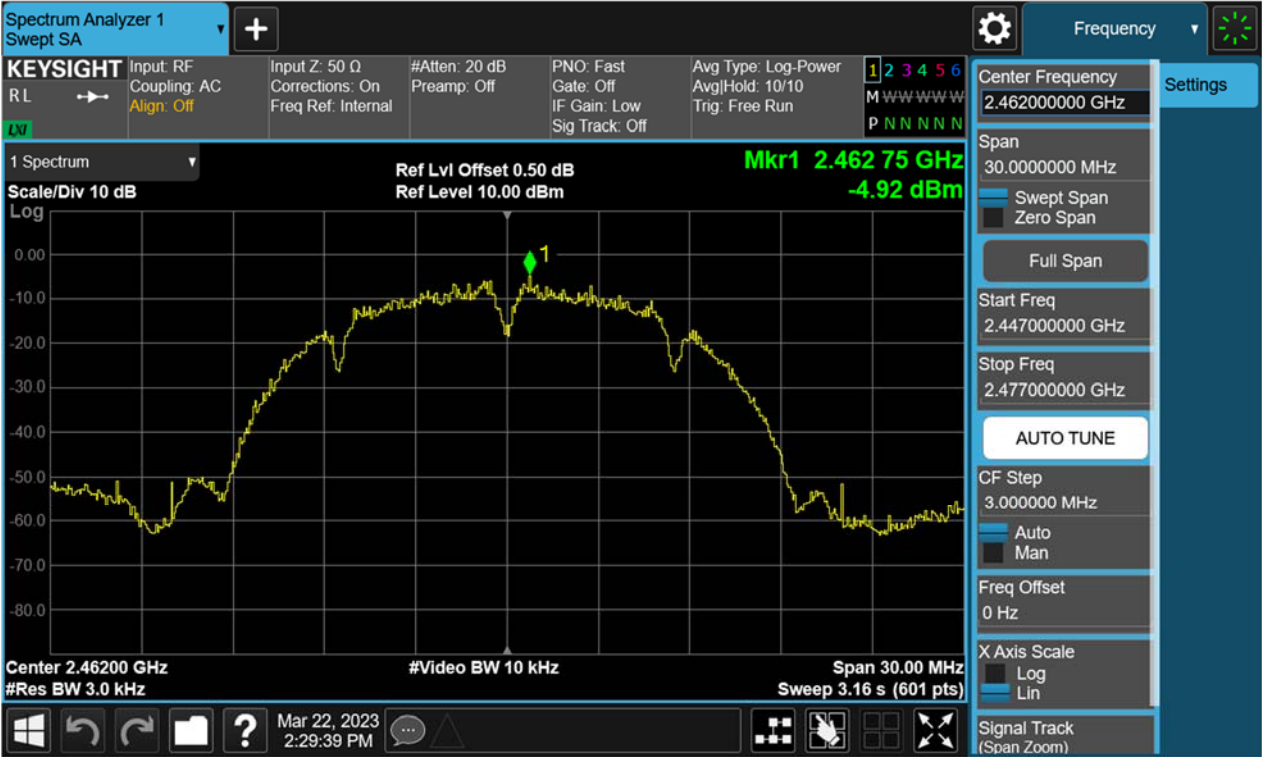
Figure 16: Power Spectral Density, 802.11g, 2412MHz
