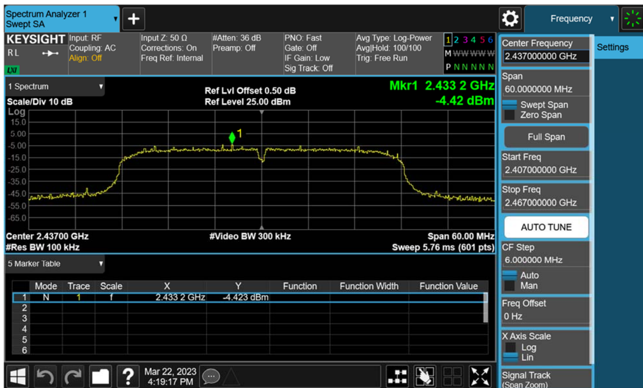
Figure 35: Conducted Spurious Emission & Authorized-band band-edge, 802.11n(HT40), 2437MHz Carrier Level
