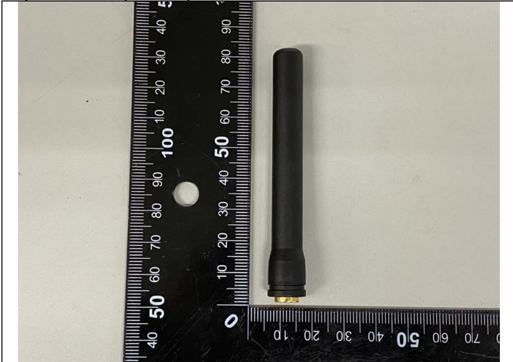
Dipole Antenna(3.96 dBi)
