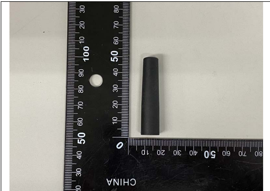
Dipole Antenna(3.14 dBi)
