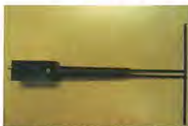
Figure 1 – MVG COMOSAR Validation Dipole
