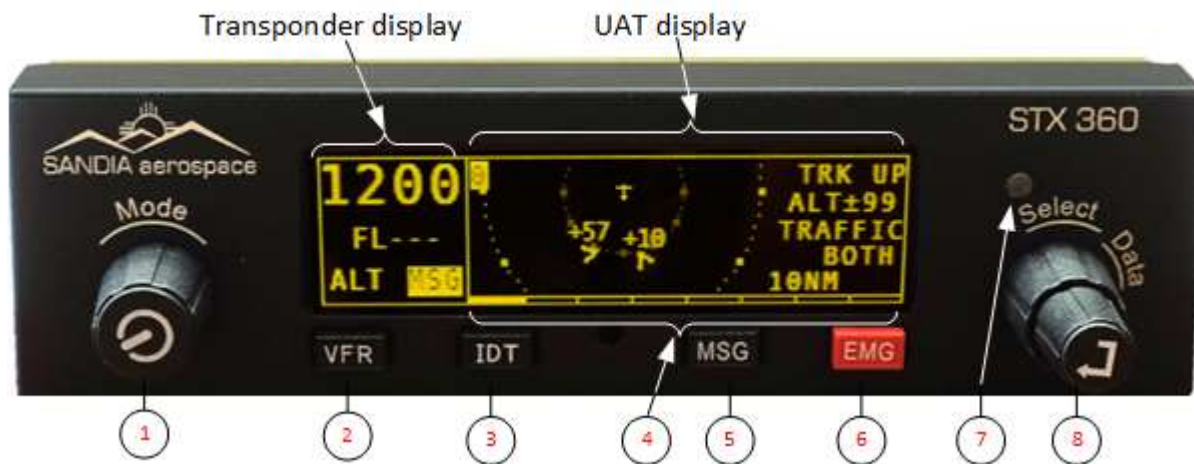
Figure 21: STX 360 front panel functionality
