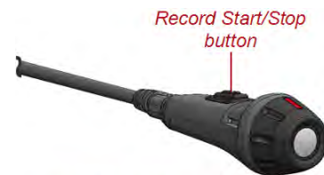
VISTA XLT head-mounted camera sensor
