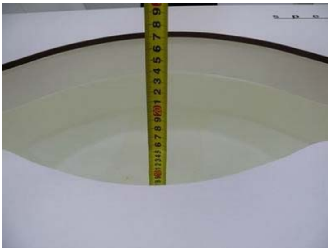
Picture 4: Liquid depth in the flat Phantom (2450 MHz, 15.3cm depth)
