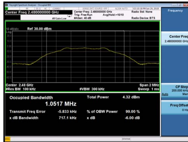
BLE Carrier frequency (MHz): 2480
