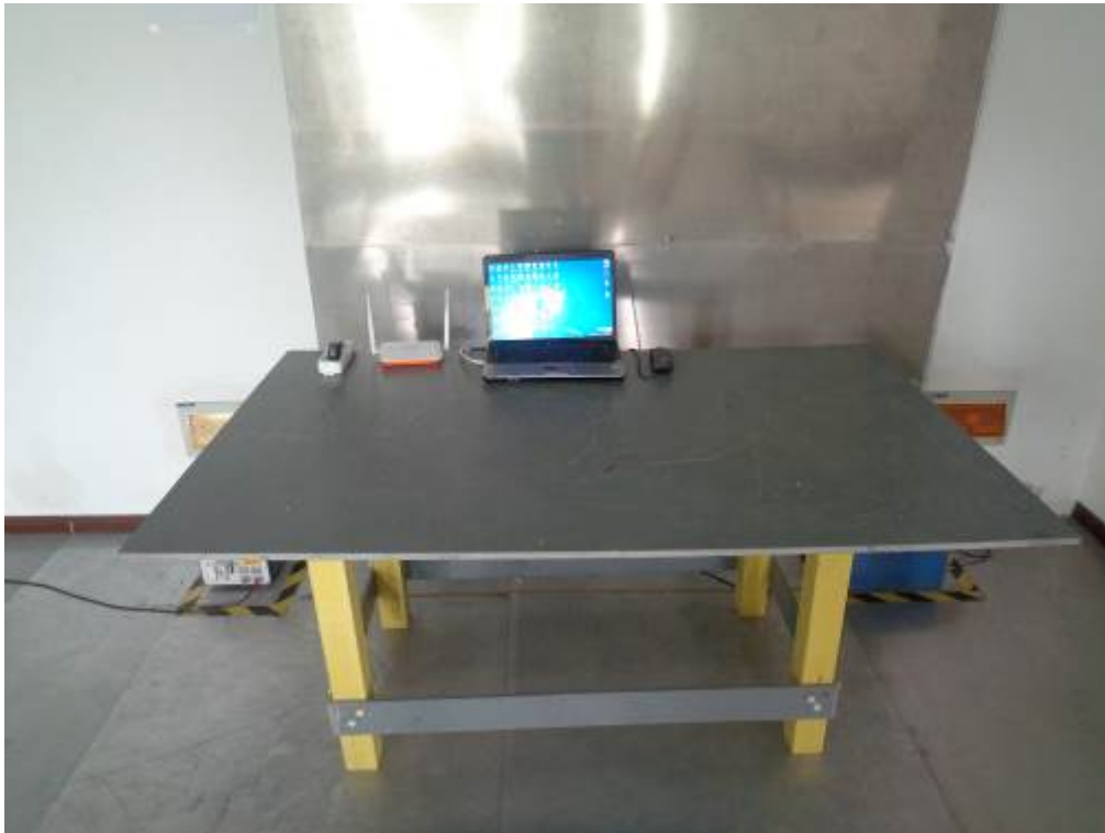
Conducted Emissions Test Setup Front View
