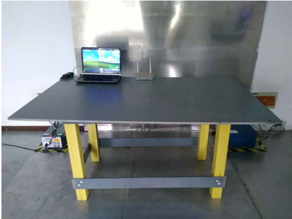
Conducted Emissions Test Setup Front View-Adapter: PSAA06A-120
