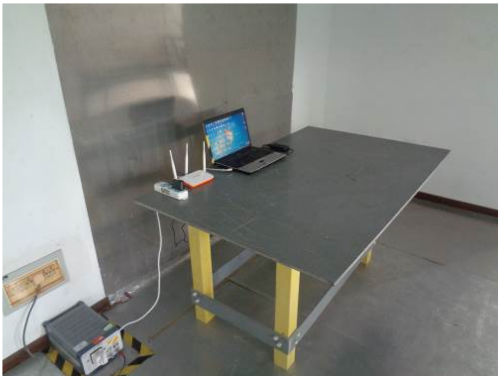
Conducted Emissions Test Setup – Side View
