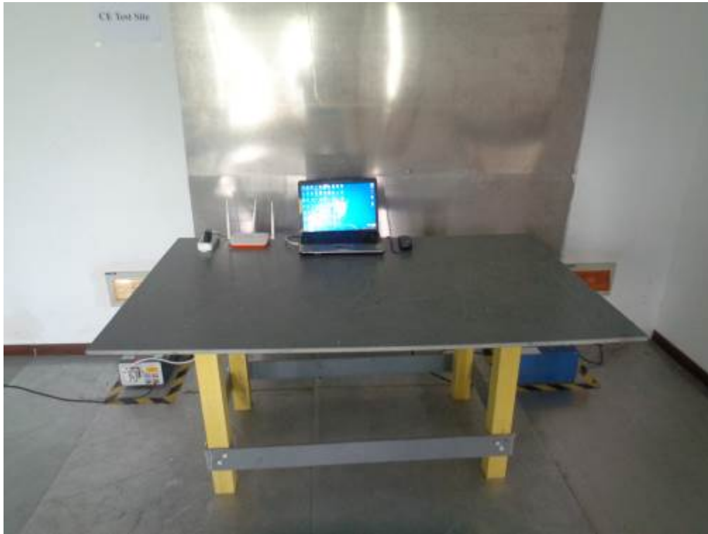
Conducted Emissions Test Setup – Front View
