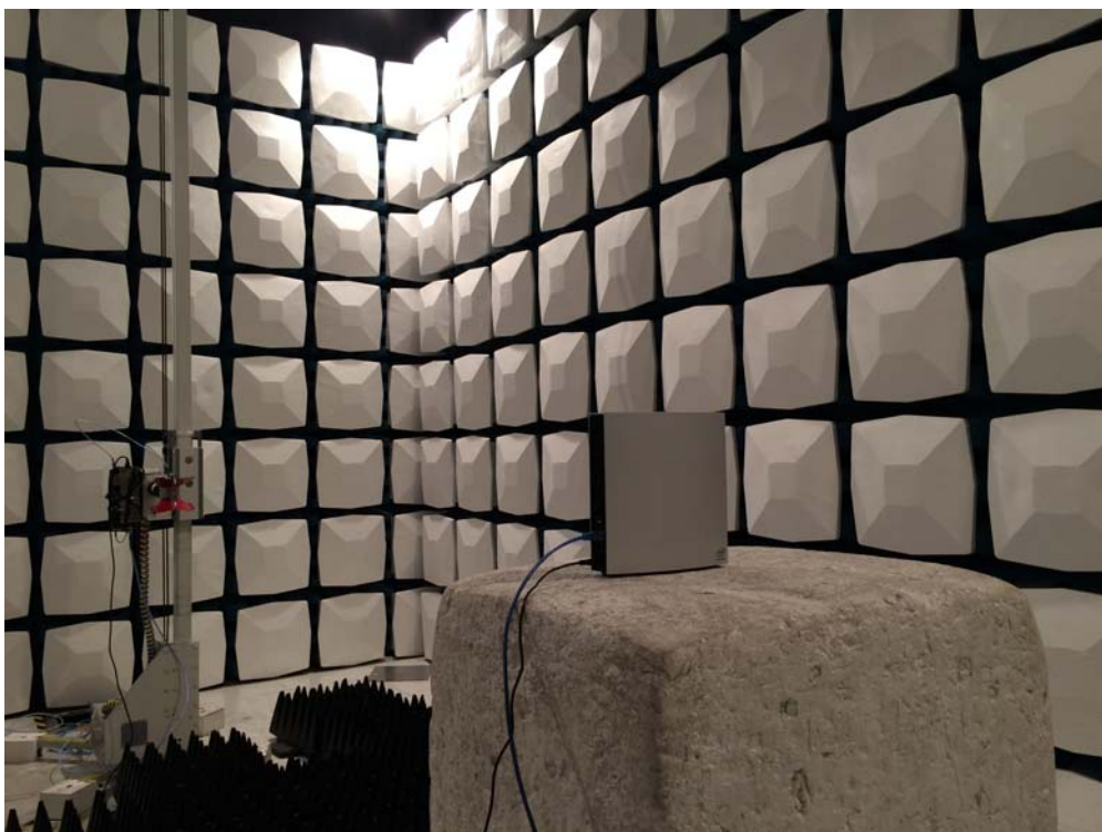
Description: Radiated Emission Test Setup for 1~18GHz
