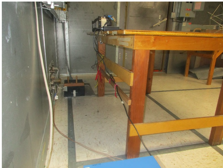
Figure 8: Back – Power Line Conducted
