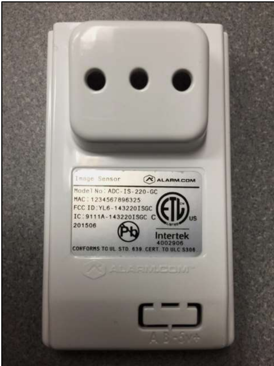
Photograph 1: ID Label & Location
