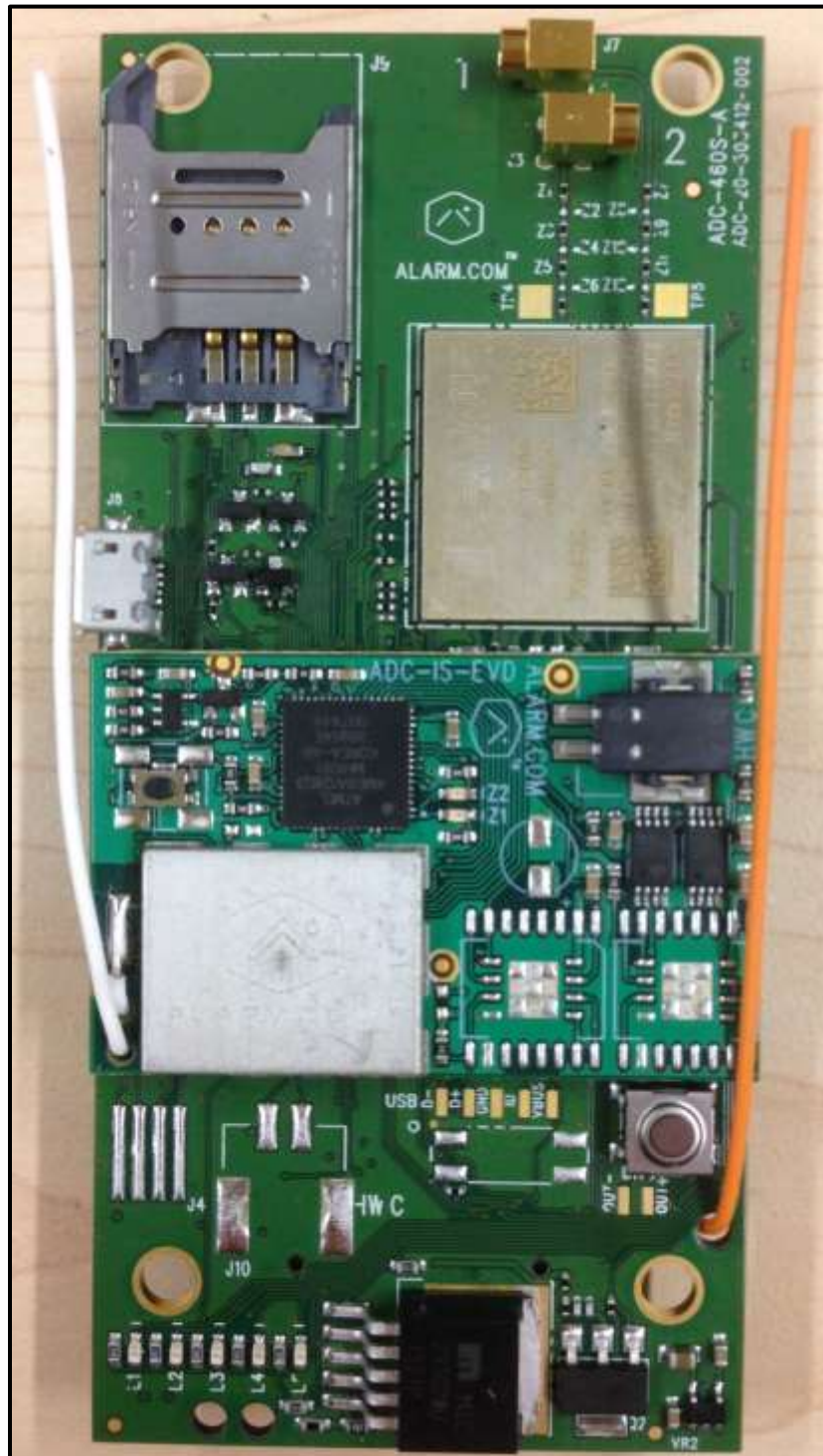
Photograph 11: PCB Top with ISDB
