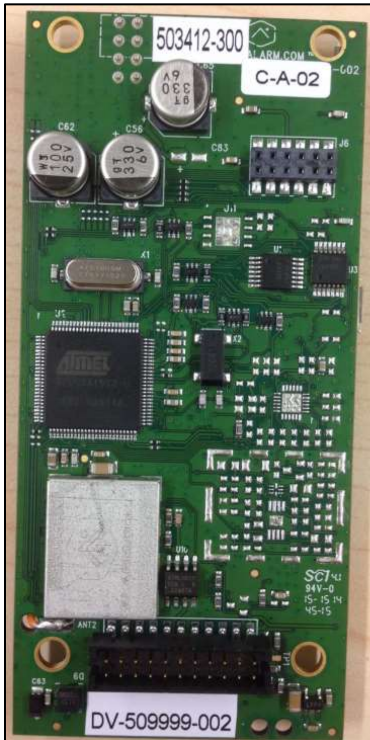
Photograph 19: PCB Bottom with Shield
