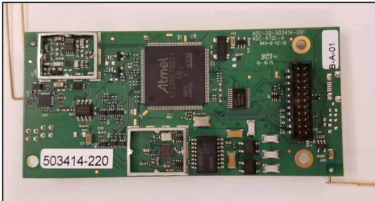
Photograph 13: Module Bottom View – No Shields
