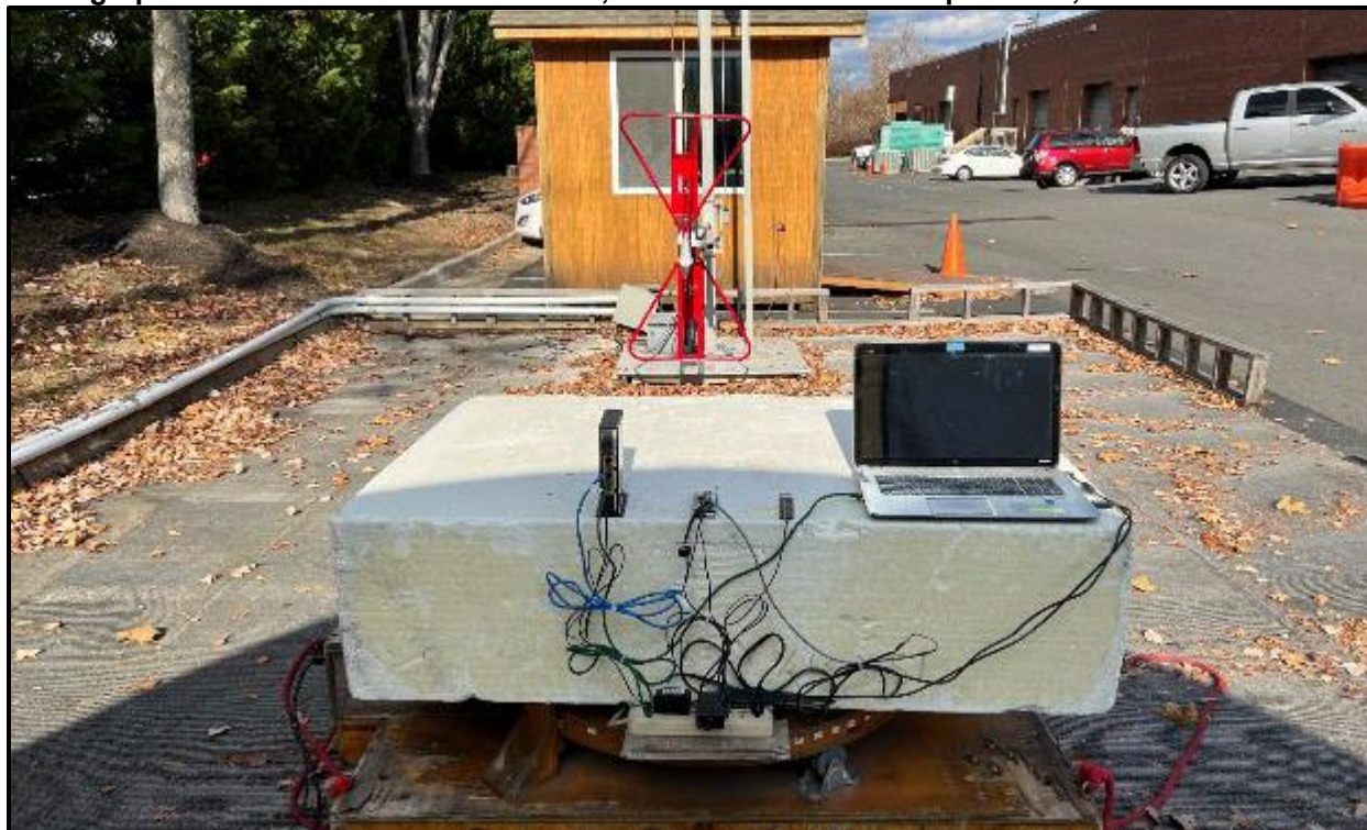
Photograph 8: Radiated Emissions, Unintentional Test Setup <1 GHz, Rear View
