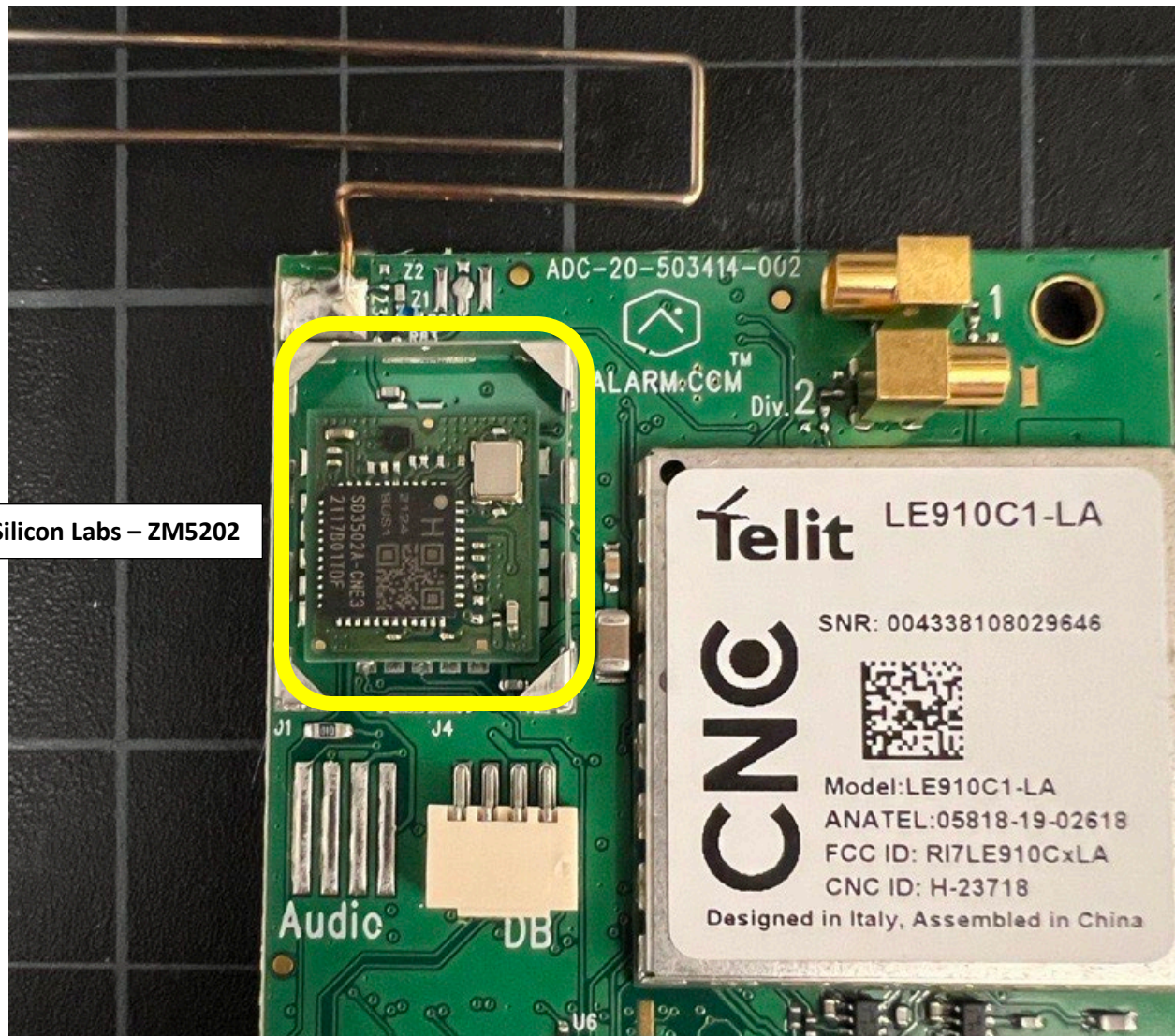
ADC-SEM-300 – Photo 10 – Top PCB – Top View No Shields; Z-Wave Module Zoomed
