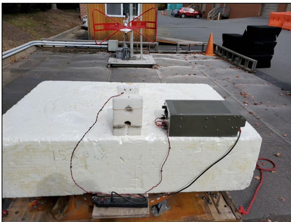
Photograph 2: Radiated Emissions Testing – Back View (Unintentional Emissions, <1 GHz)
