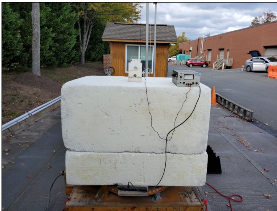
Photograph 4: Radiated Emissions Testing – Back View (Spurious Emissions, >1 GHz)
