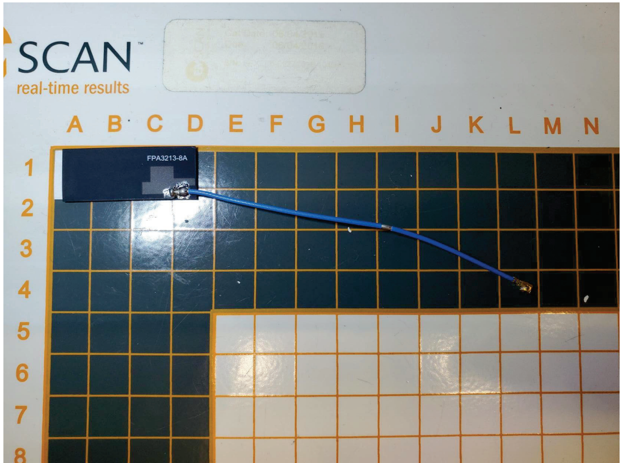
Inpaq Antenna (RFFPA321309IMRB402) [LoRa option 1]
