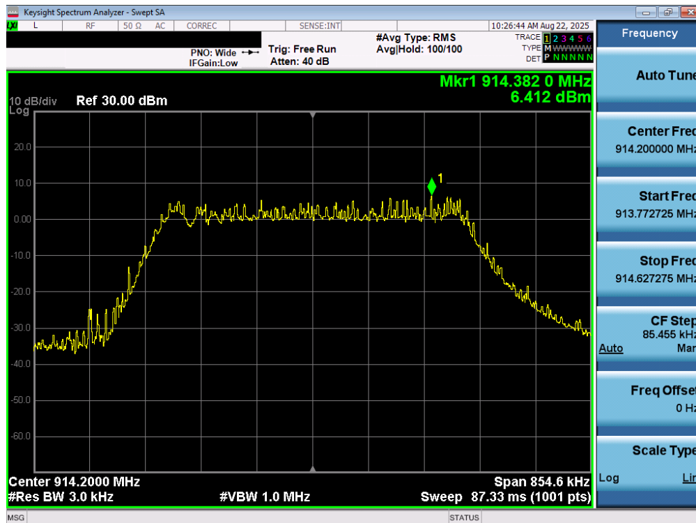
Plot 7-20. Power Spectral Density Measurements (500kHz DTS Mode – Ch.71)
