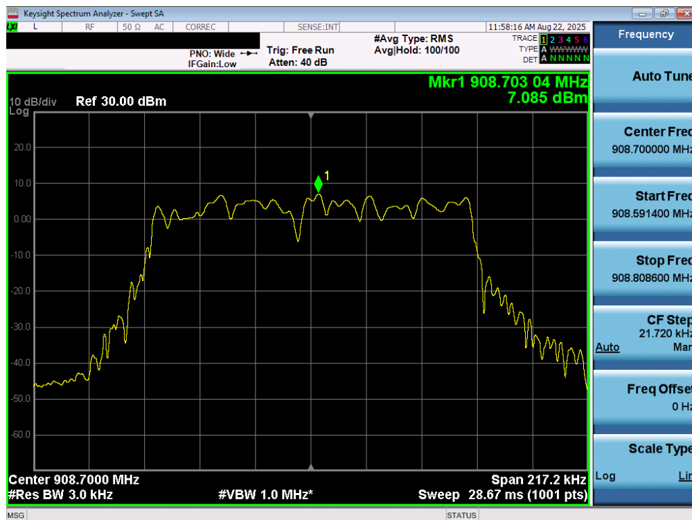
Plot 7-17. Power Spectral Density Measurements (125kHz FHSS/Hybrid Mode – Ch.32 )
