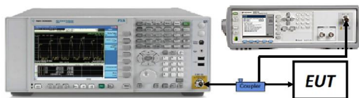
Figure 7-8. Test Instrument & Measurement Setup
