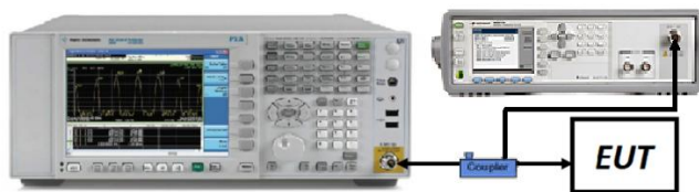
Figure 7-2. Test Instrument & Measurement Setup
