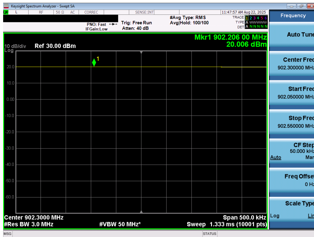
Plot 7-13. Peak Conducted Power (125kHz Hybrid Mode – Ch. 0)
