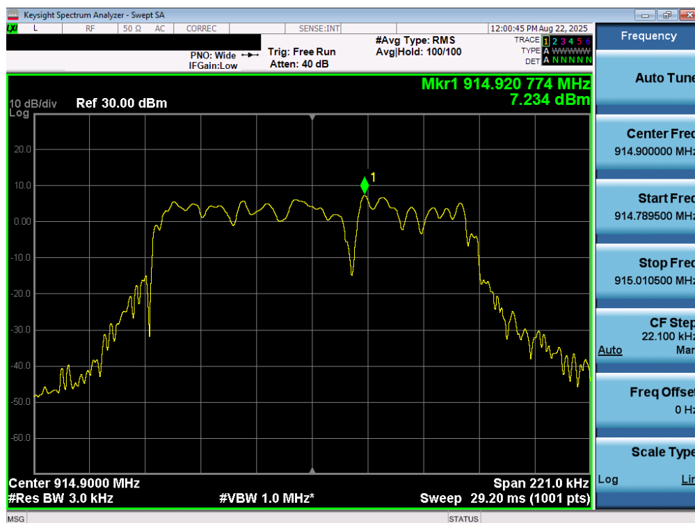
Plot 7-18. Power Spectral Density Measurements (125kHz FHSS/Hybrid Mode – Ch.63)
