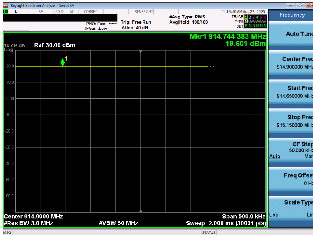
Plot 7-9. Peak Conducted Power (125kHz FHSS Mode – Ch. 63)
