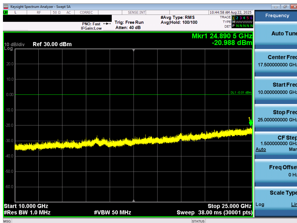
Plot 7-40. Conducted Spurious Plot (LoRa, 500kHz DTS Mode – Ch. 64)
