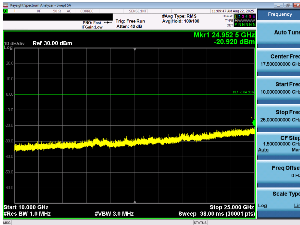
Plot 7-34. Conducted Spurious Plot (LoRa, 125kHz FHSS Mode – Ch. 0)
