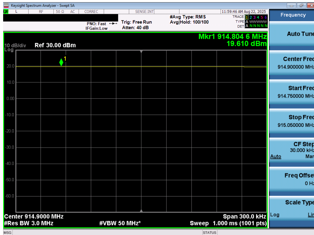
Plot 7-15. Peak Conducted Power (125kHz Hybrid Mode – Ch. 63)
