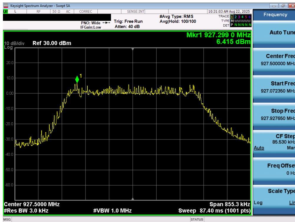
Plot 7-21. Power Spectral Density Measurements (500kHz DTS Mode – Ch. 7)
