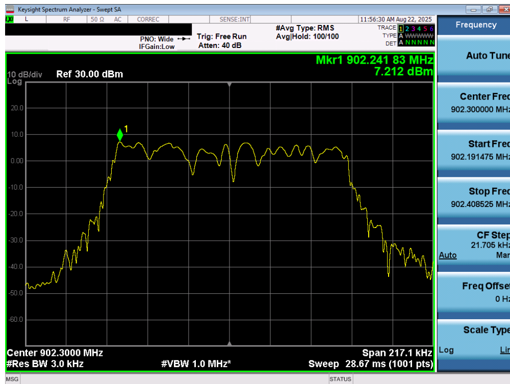
Plot 7-16. Power Spectral Density Measurements (125kHz FHSS/Hybrid Mode – Ch. 0)
