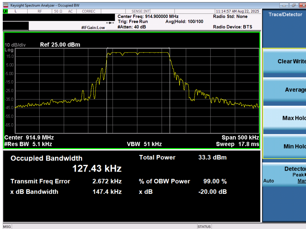
Plot 7-3. 20dB Bandwidth Plot (LoRa, 125kHz FHSS/Hybrid Mode – Ch. 63)
