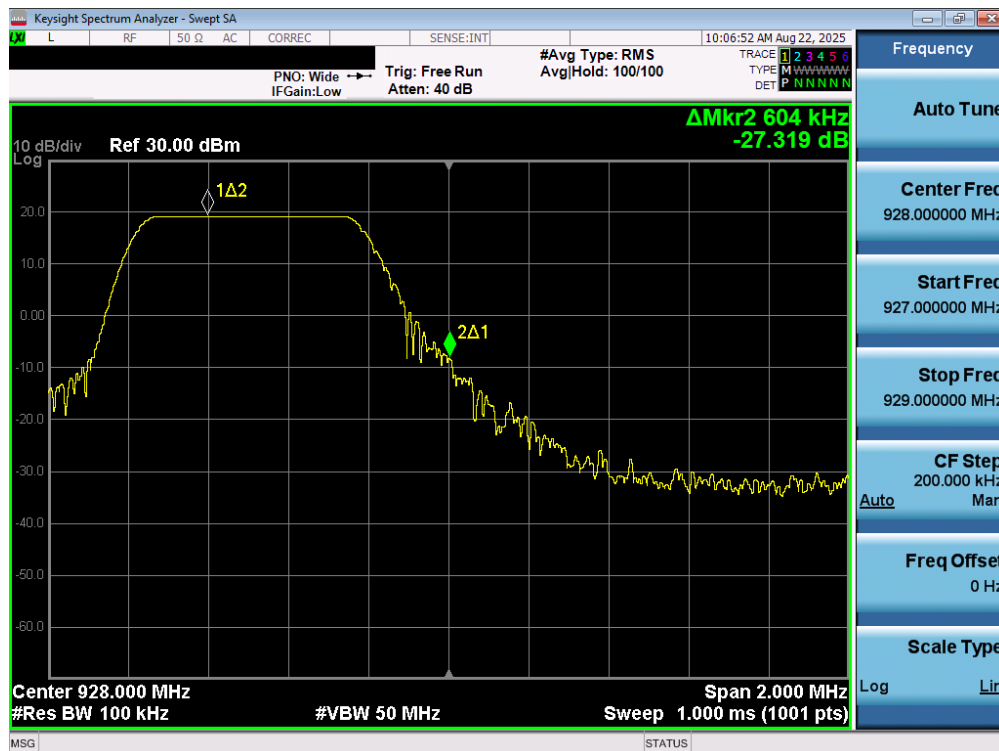
Plot 7-27. Band Edge Plot (LoRa, 500kHz DTS Mode – Ch. 7)
