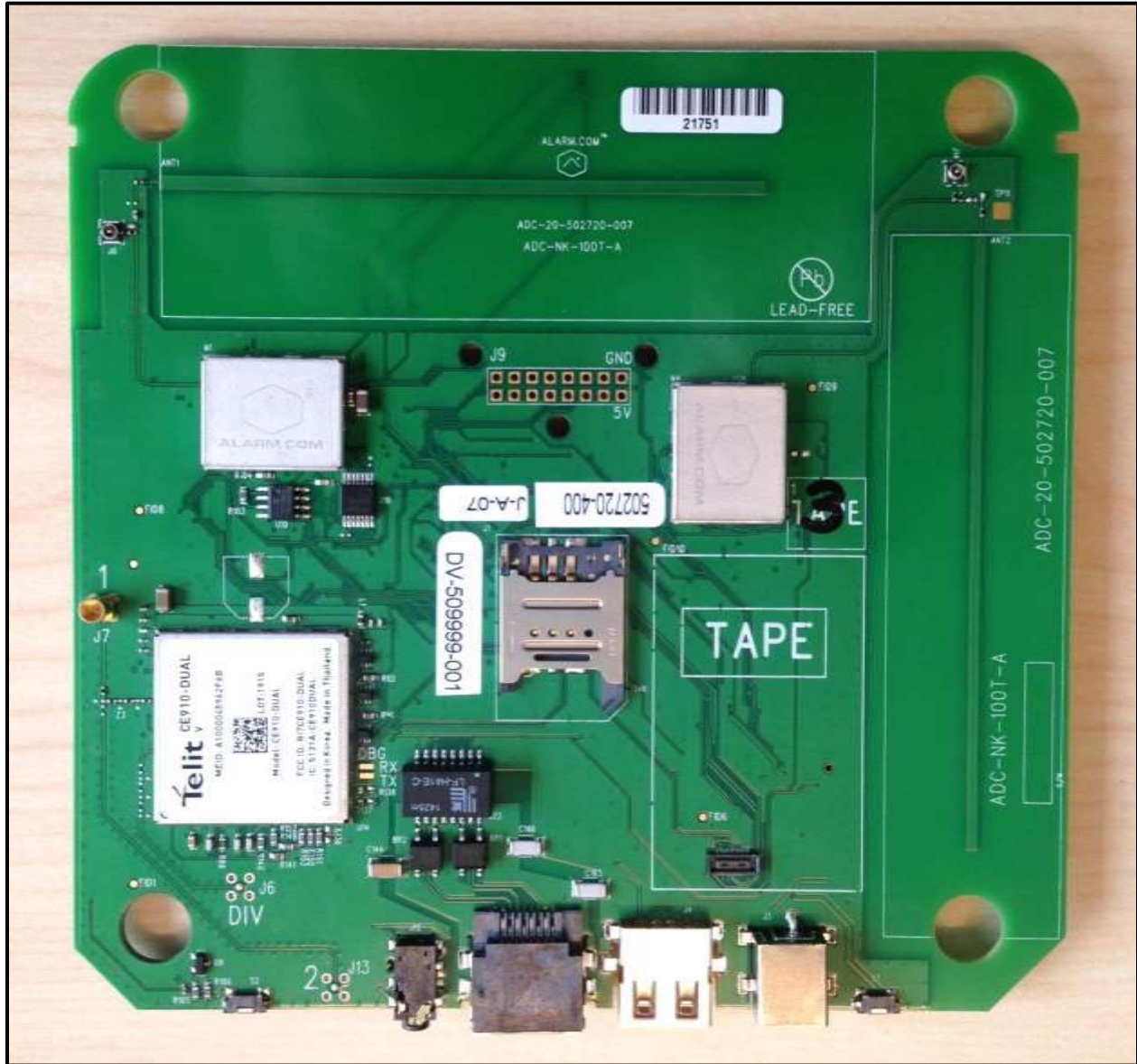
Photograph 18: Fully Populated PCB – Top View with Shields
