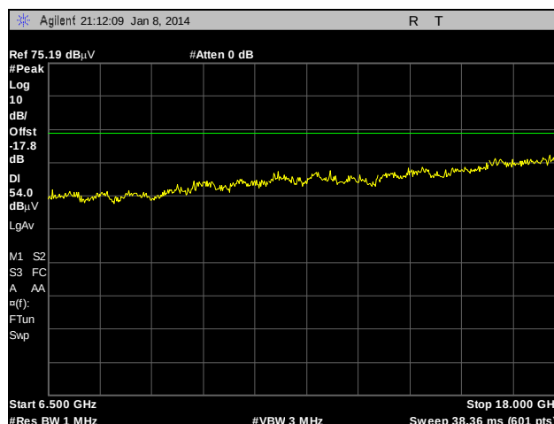
Plot 105. Radiated Spurious Emissions, Internal Antenna, 802.11n 40 MHz, 5310 MHz, 6.5 GHz – 18 GHz, Peak under Average
