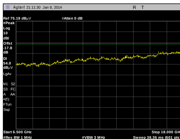
Plot 102. Radiated Spurious Emissions, Internal Antenna, 802.11n 40 MHz, 5270 MHz, 6.5 GHz – 18 GHz, Peak under Average
