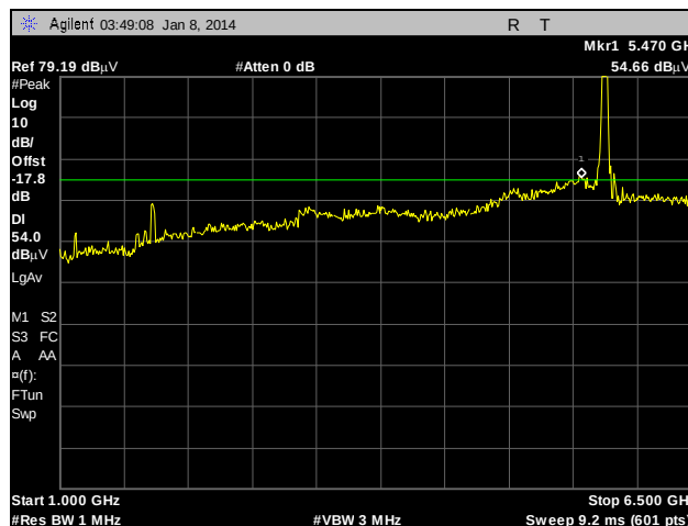
Plot 212. Radiated Spurious Emissions, External Antenna, 802.11n 40 MHz, 5670 MHz, 1 GHz – 6.5 GHz, Peak under Average
