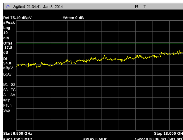
Plot 165. Radiated Spurious Emissions, External Antenna, 802.11a, 5300 MHz, 6.5 GHz – 18 GHz, Peak under Average
