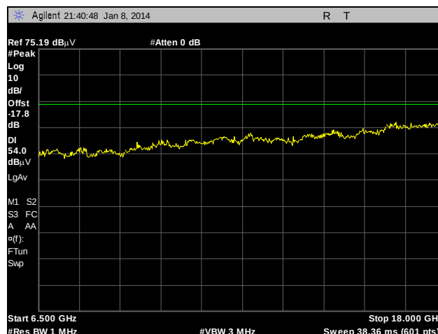
Plot 156. Radiated Spurious Emissions, External Antenna, 802.11n 40 MHz, 5190 MHz, 6.5 GHz – 18 GHz, Peak under Average
