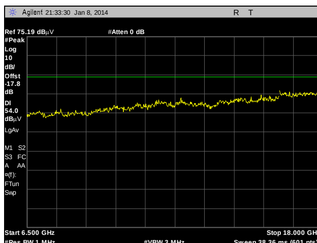
Plot 141. Radiated Spurious Emissions, External Antenna, 802.11a, 5200 MHz, 6.5 GHz – 18 GHz, Peak under Average
