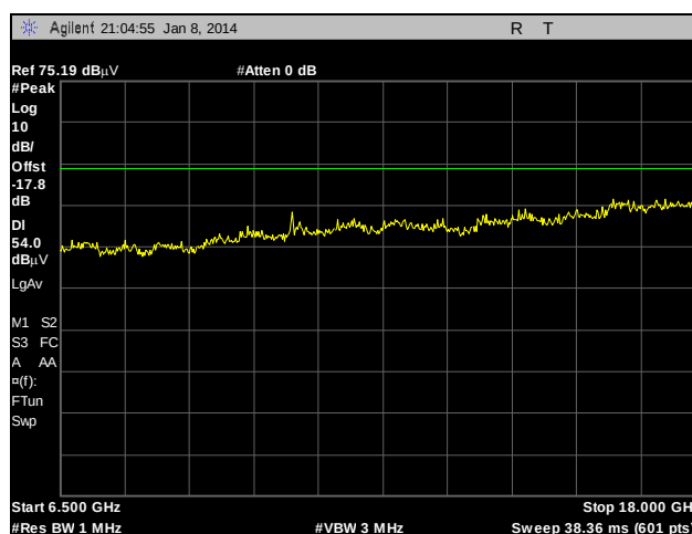
Plot 99. Radiated Spurious Emissions, Internal Antenna, 802.11n 20 MHz, 5320 MHz, 6.5 GHz – 18 GHz, Peak under Average
