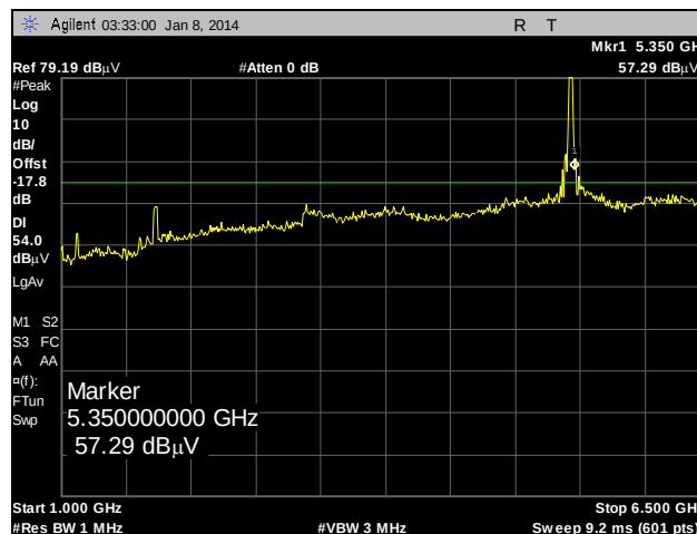
Plot 176. Radiated Spurious Emissions, External Antenna, 802.11n 20 MHz, 5320 MHz, 1 GHz – 6.5 GHz, Peak under Average
