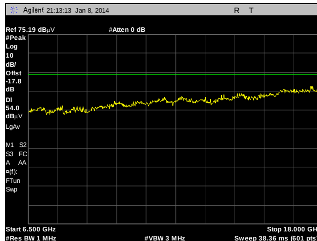
Plot 131. Radiated Spurious Emissions, Internal Antenna, 802.11n 40 MHz, 5550 MHz, 6.5 GHz – 18 GHz, Peak under Average
