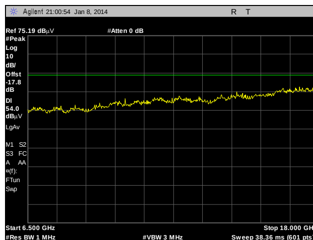
Plot 69. Radiated Spurious Emissions, Internal Antenna, 802.11n 20 MHz, 5180 MHz, 6.5 GHz – 18 GHz, Peak under Average
