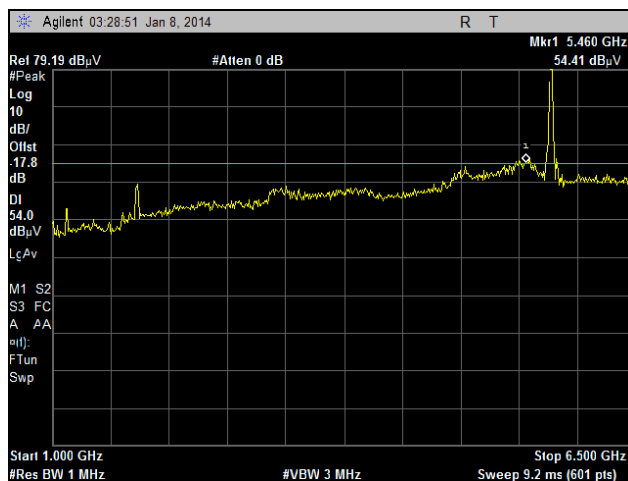
Plot 202. Radiated Spurious Emissions, External Antenna, 802.11n 20 MHz, 5700 MHz, 1 GHz – 6.5 GHz, Peak under Average
