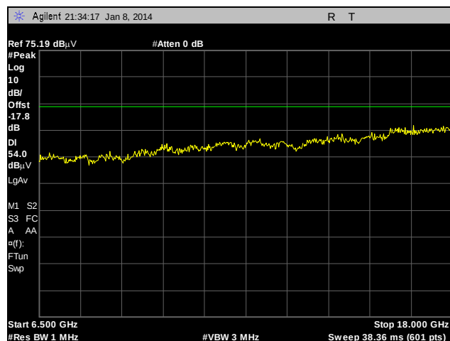
Plot 162. Radiated Spurious Emissions, External Antenna, 802.11a, 5260 MHz, 6.5 GHz – 18 GHz, Peak under Average
