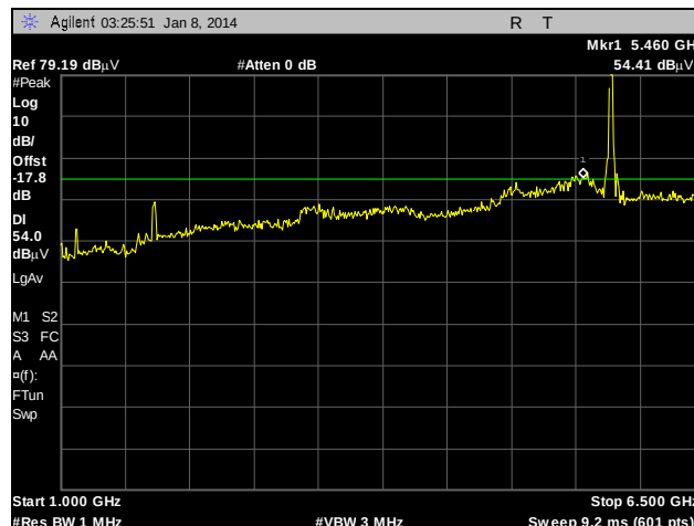
Plot 192. Radiated Spurious Emissions, External Antenna, 802.11a, 5700 MHz, 1 GHz – 6.5 GHz, Peak under Average
