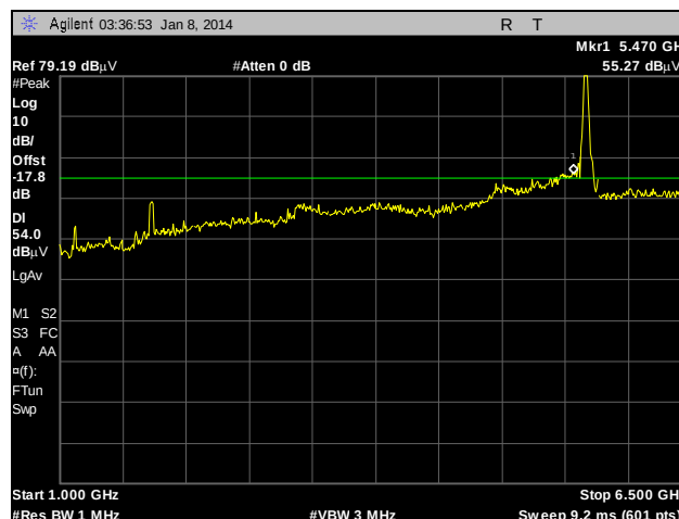
Plot 198. Radiated Spurious Emissions, External Antenna, 802.11n 20 MHz, 5580MHz, 1 GHz – 6.5 GHz, Peak under Average
