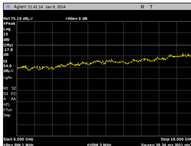
Plot 159. Radiated Spurious Emissions, External Antenna, 802.11n 40 MHz, 5230 MHz, 6.5 GHz – 18 GHz, Peak under Average
