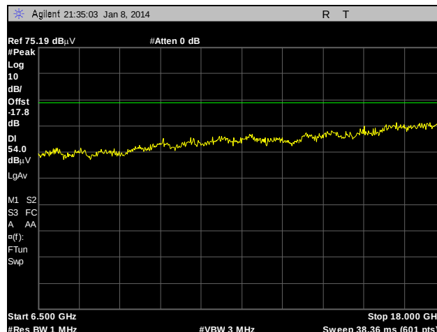
Plot 168. Radiated Spurious Emissions, External Antenna, 802.11a, 5320 MHz, 6.5 GHz – 18 GHz, Peak under Average
