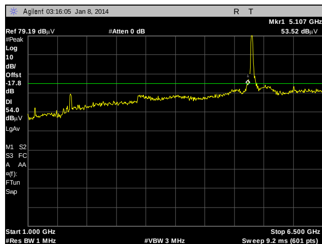
Plot 137. Radiated Spurious Emissions, External Antenna, 802.11a, 5180 MHz, 1 GHz – 6.5 GHz, Peak under Average
