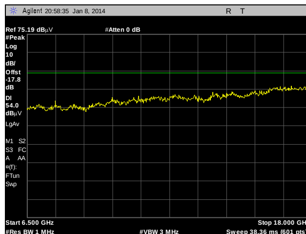
Plot 108. Radiated Spurious Emissions, Internal Antenna, 802.11a, 5500 MHz, 6.5 GHz – 18 GHz, Peak under Average
