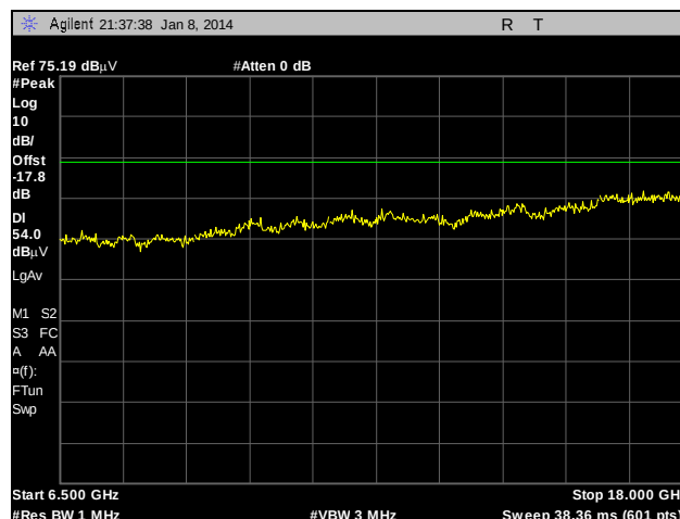
Plot 153. Radiated Spurious Emissions, External Antenna, 802.11n 20 MHz, 5240 MHz, 6.5 GHz – 18 GHz, Peak under Average
