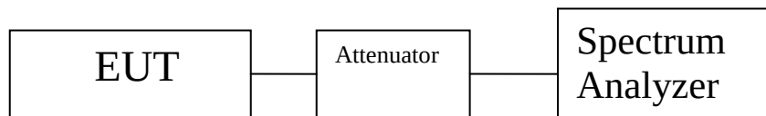
Figure 2. Power Output Test Setup
