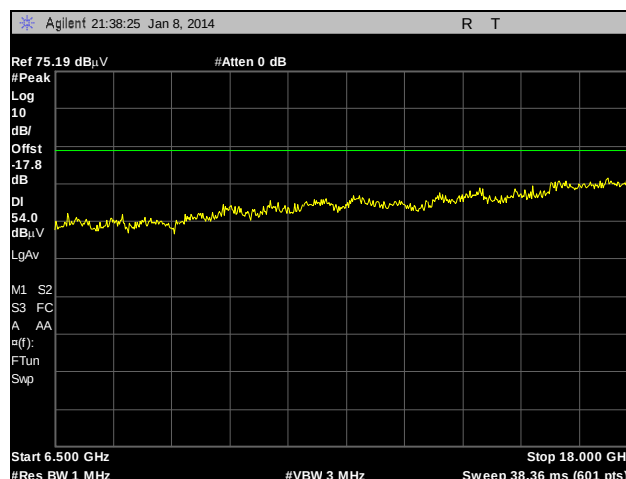
Plot 174. Radiated Spurious Emissions, External Antenna, 802.11n 20 MHz, 5300 MHz, 6.5 GHz – 18 GHz, Peak under Average
