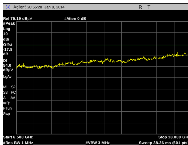
Plot 66. Radiated Spurious Emissions, Internal Antenna, 802.11a, 5240 MHz, 6.5 GHz – 18 GHz, Peak under Average
