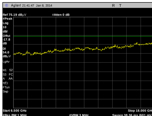
Plot 180. Radiated Spurious Emissions, External Antenna, 802.11n 40 MHz, 5270 MHz, 6.5 GHz – 18 GHz, Peak under Average
