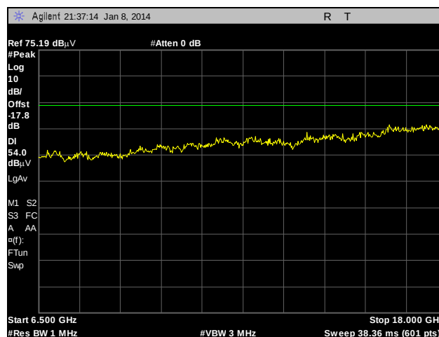
Plot 150. Radiated Spurious Emissions, External Antenna, 802.11n 20 MHz, 5200 MHz, 6.5 GHz – 18 GHz, Peak under Average
