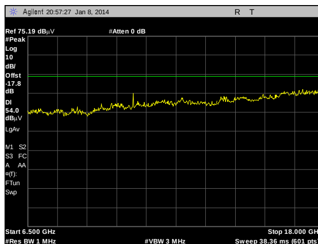
Plot 87. Radiated Spurious Emissions, Internal Antenna, 802.11a, 5300 MHz, 6.5 GHz – 18 GHz, Peak under Average
