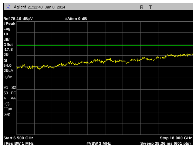
Plot 138. Radiated Spurious Emissions, External Antenna, 802.11a, 5180 MHz, 6.5 GHz – 18 GHz, Peak under Average
