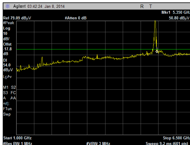
Plot 179. Radiated Spurious Emissions, External Antenna, 802.11n 40 MHz, 5270 MHz, 1 GHz – 6.5 GHz, Peak under Average
