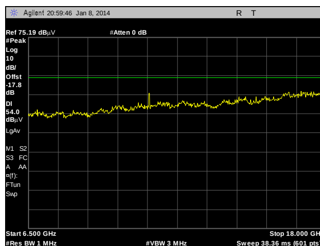
Plot 111. Radiated Spurious Emissions, Internal Antenna, 802.11a, 5580 MHz, 6.5 GHz – 18 GHz, Peak under Average
