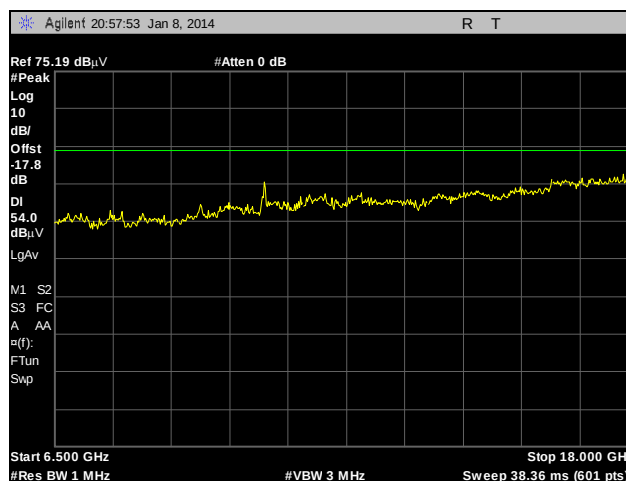
Plot 90. Radiated Spurious Emissions, Internal Antenna, 802.11a, 5320 MHz, 6.5 GHz – 18 GHz, Peak under Average
