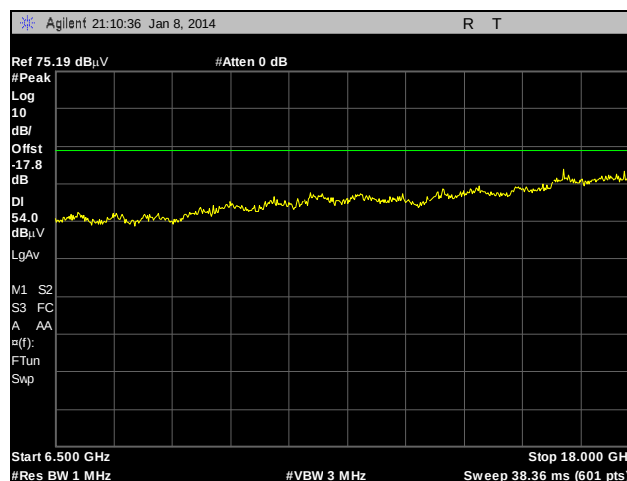
Plot 78. Radiated Spurious Emissions, Internal Antenna, 802.11n 40 MHz, 5190 MHz, 6.5 GHz – 18 GHz, Peak under Average
