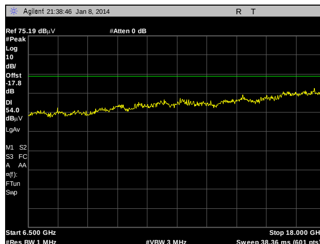
Plot 177. Radiated Spurious Emissions, External Antenna, 802.11n 20 MHz, 5320 MHz, 6.5 GHz – 18 GHz, Peak under Average
