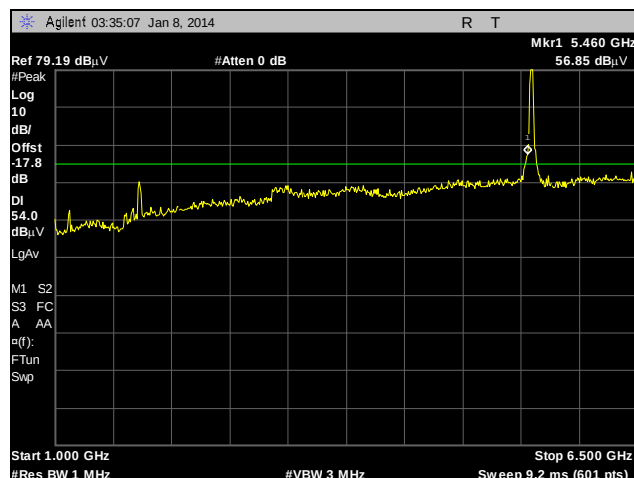
Plot 195. Radiated Spurious Emissions, External Antenna, 802.11n 20 MHz, 5500 MHz, 1 GHz – 6.5 GHz, Peak under Average
