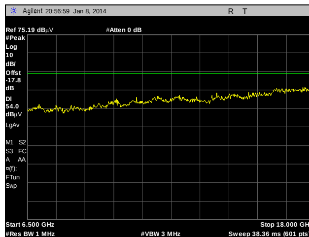
Plot 84. Radiated Spurious Emissions, Internal Antenna, 802.11a, 5260 MHz, 6.5 GHz – 18 GHz, Peak under Average
