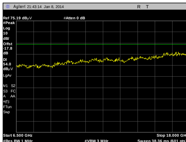
Plot 213. Radiated Spurious Emissions, External Antenna, 802.11n 40 MHz, 5670 MHz, 6.5 GHz – 18 GHz, Peak under Average
