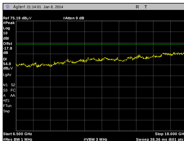
Plot 135. Radiated Spurious Emissions, Internal Antenna, 802.11n 40 MHz, 5670 MHz, 6.5 GHz – 18 GHz, Peak under Average
